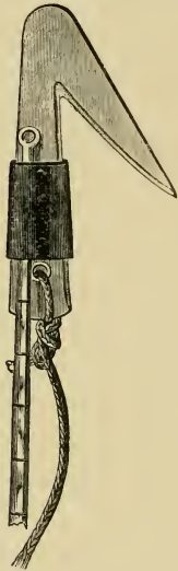
The releaser, for cutting branches.
