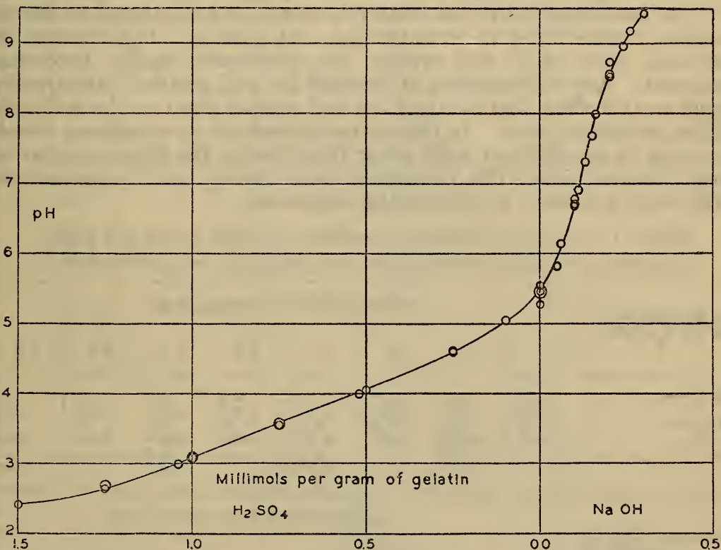
FIGURE 2.—Titration curve of isoelectric gelatin used in experiments, at a concentration of 1.00 g per 100 ml
