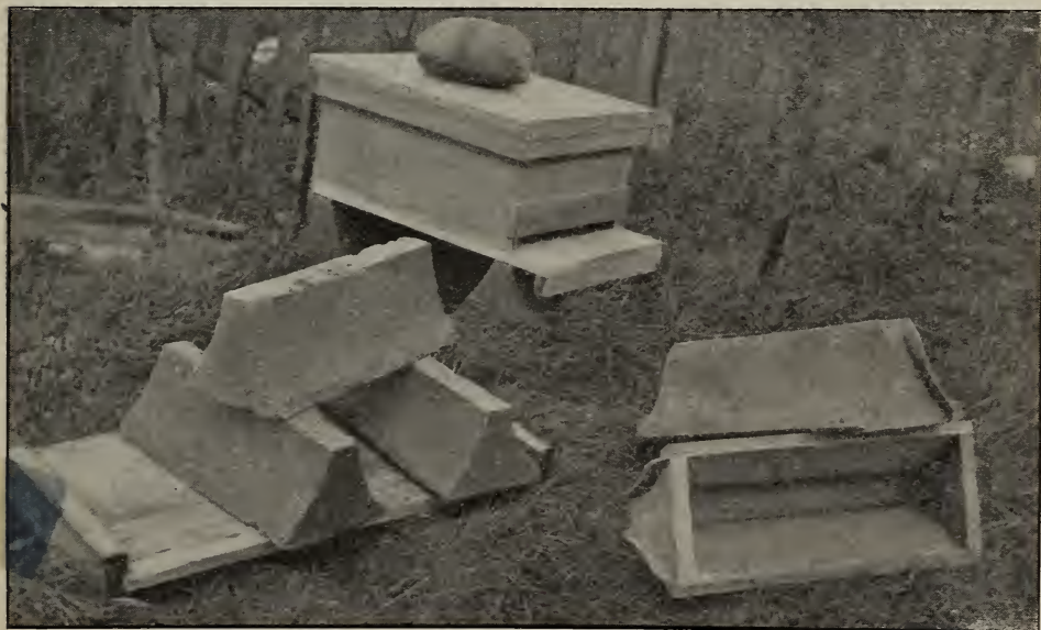
FIG. 1.—C. V. Rice's concrete hive-stands, and form for making them.
