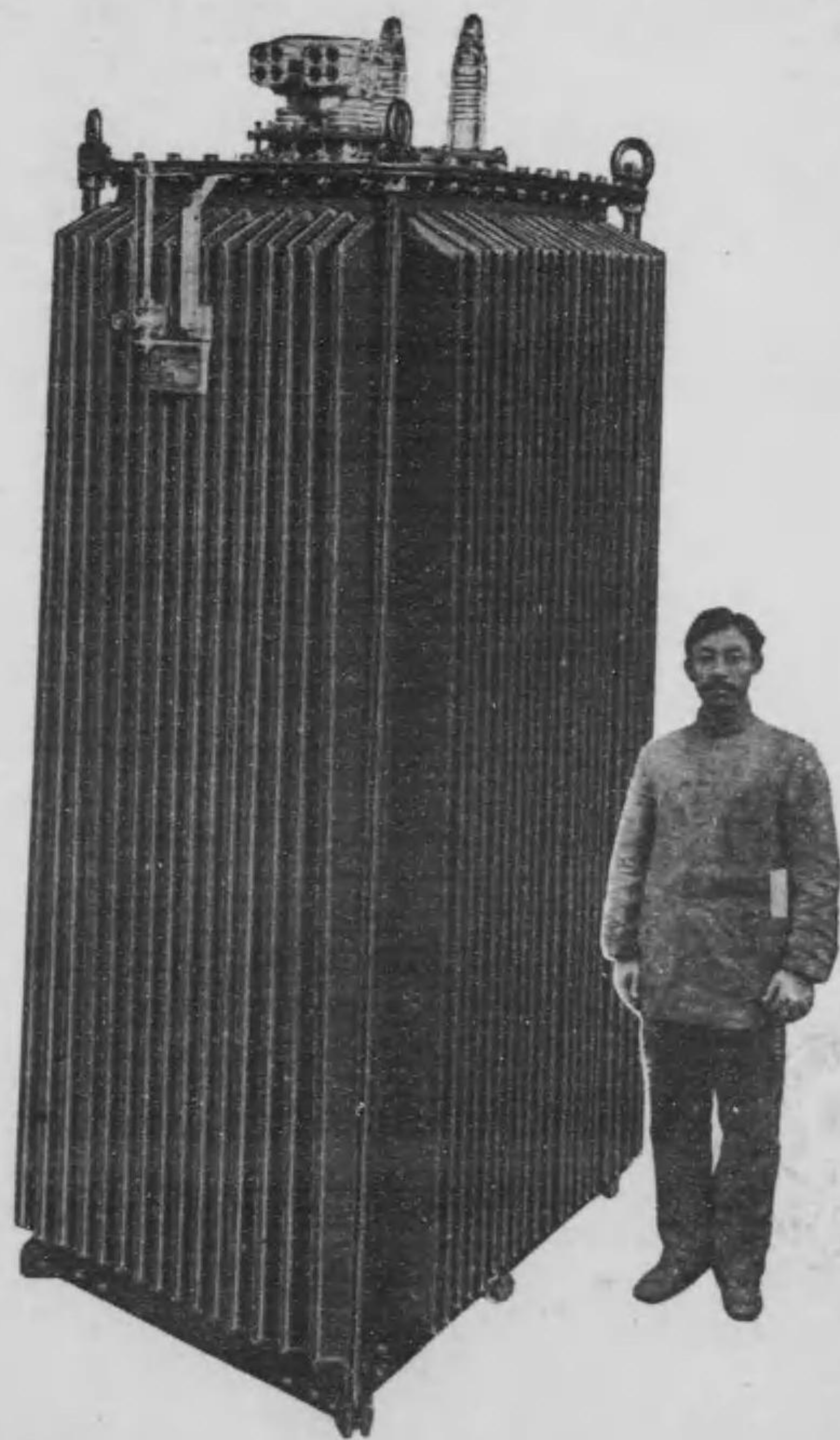
Single phase, 50 cycles, 30,000/3,500 V. 1,000 K.V.A. Oil Cooling TRANSFORMER.
