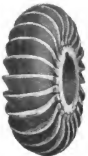
Convex and Concave Cutters with Plain Milling Cutter Type of Teeth
