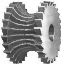
Formed Cutter. Teeth can be sharpened without changing Contour
