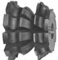
Formed Cutter. Teeth can be sharpened without changing Contour
