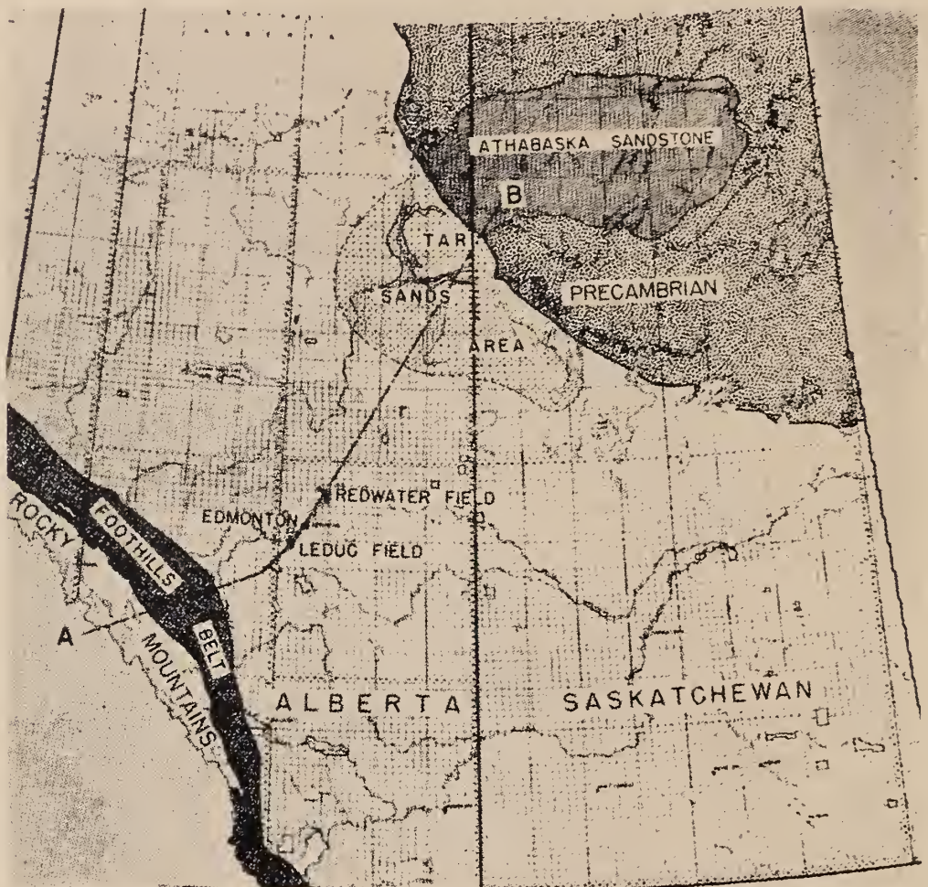
Fig. 1. Index map of Alberta and Saskatchewan showing areal relationship between oil sands of Lower Cretaceous age in sedimentary basin area and Precambrian "Athabasca sandstone" on Canadian shield. AB indicates position of cross-section (Fig. 2) which begins at B in Athabasca sandstone on the Shield, and passes through the oil sands, Redwater and Leduc coral-reef oil pools, near Edmonton, and thence through deeper part of Alberta syncline, Foothills Belt, and Rocky Mountains at A.
