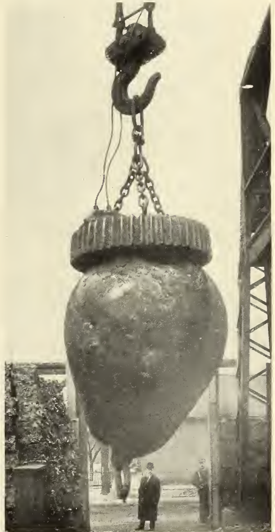
ELECTRO-MAGNET LIFTING A "SKULL-CRACKER" WEIGHING 13,000 POUNDS.
