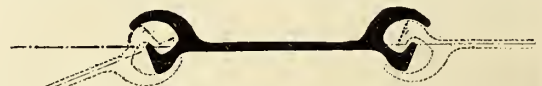
TOP VIEW OF A SHEET-PILE SHOWING BY DOTTED LINES HOW IT INTERLOCKS WITH PILES AT EACH SIDE.
