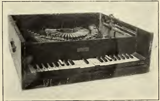
AN EARLY FORM OF TYPE-WRITER, HAVING THE PIANO KEYBOARD.
