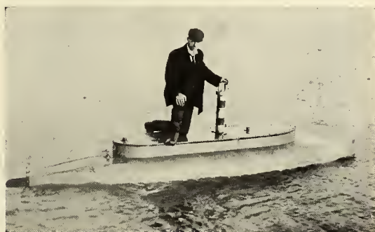
THE GARDNER TORPEDO-SUBMARINE—CONTROLLED BY SOUND WAVES.
