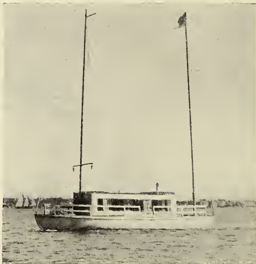
JOHN HAYS HAMMOND, JR.'S HOUSE-BOAT, DIRECTED BY WIRELESS, WHICH PRECEDED HIS WIRELESS TORPEDO-BOAT.
