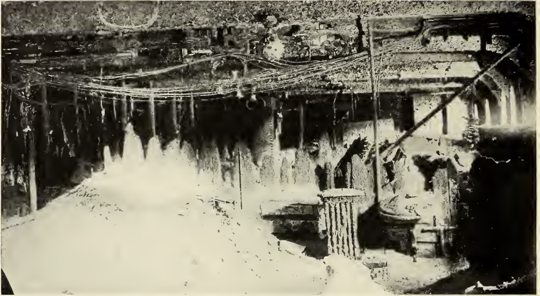
THE OFFICERS' QUARTERS ON THE "MAINE," SHOWING THE WOODEN PARTITIONS EATEN AWAY BY WORMS EXCEPT WHERE PROTECTED BY MUD. NOTE THE SHELL-INCORPORATED ELECTRIC-LIGHT BULB AT THE CEILING.
