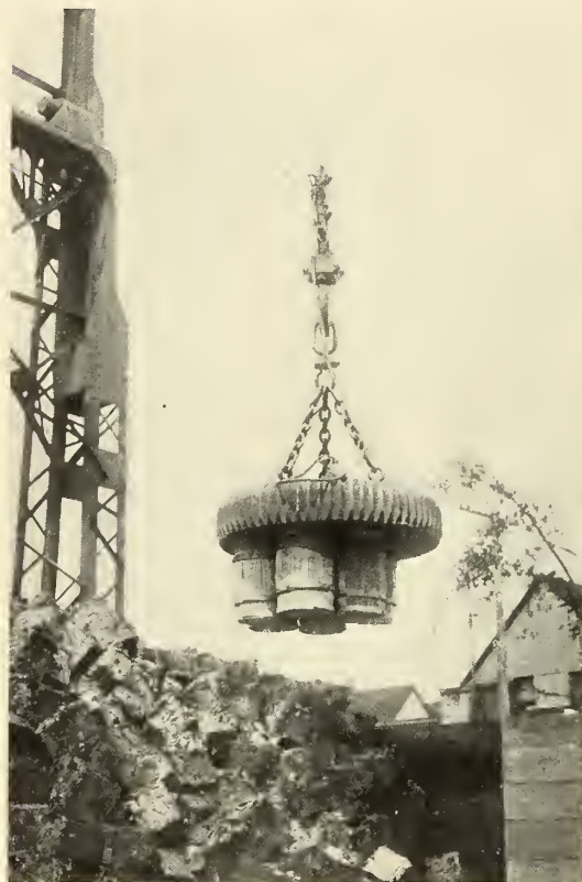
SEVEN KEGS FILLED WITH NAILS LIFTED BY AN ELECTRO-MAGNET.
