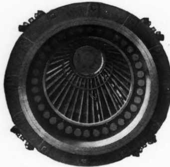
End view of revolving screen with internal protecting bars for discharging heavy lumps.
