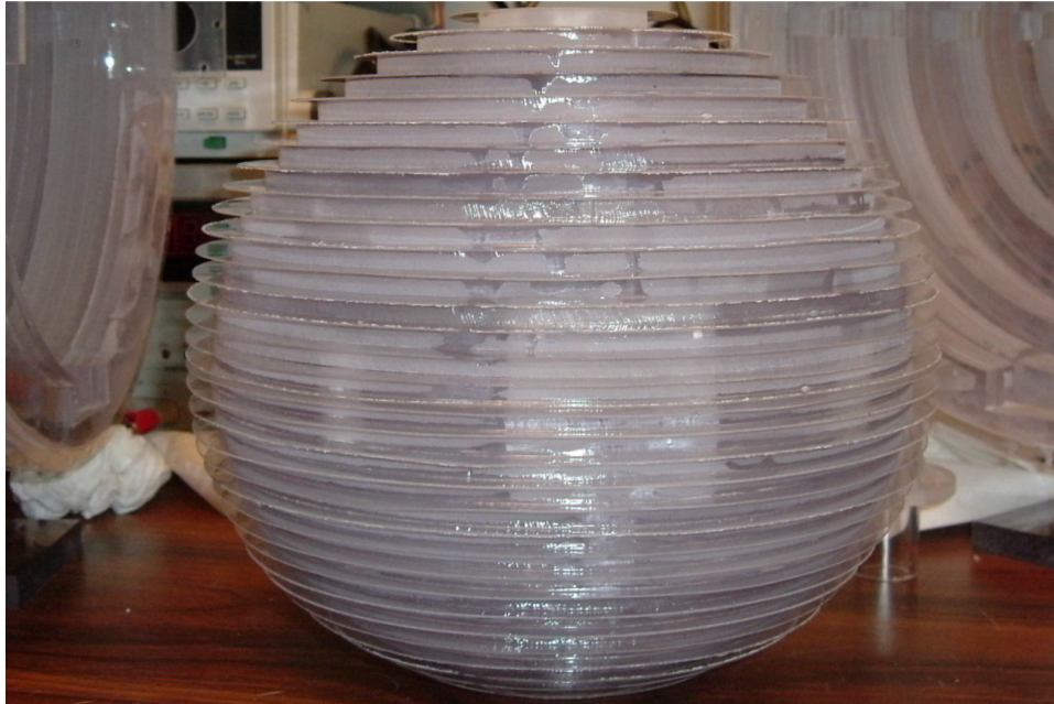
Figure C-5: The inner fluxball structure after both bonding procedures were completed.
