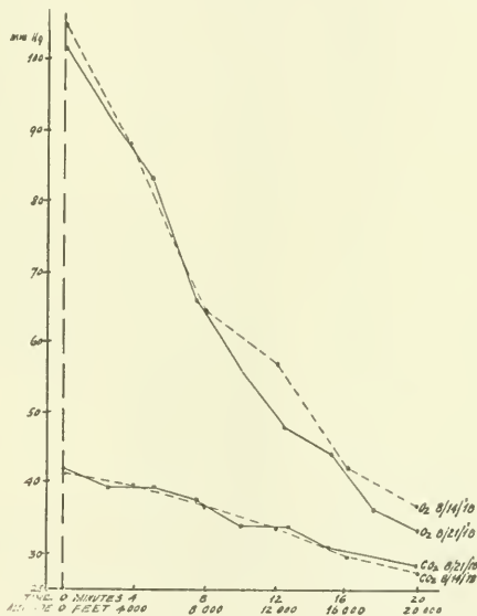
Fig. 2. Alveolar air tensions of J. B. D. taken to 352 mm. (20,000 feet) in a low pressure chamber. Dotted lines on 8/14/18 at a rate of 1000 feet a minute. Solid lines on 8/21/18 at a rate of 500 feet a minute. The carbon dioxide tension of 8/14/18 is plotted 1 mm. lower than the actual value.
