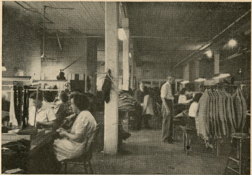
THE ABOVE PICTURE shows the type of lighting that prevailed in all four departments of the Schwob Manufacturing Company in Columbus before it was relighted in October. Bare bulbs on ceiling dropcords supplied spotty, glary general illumination that was supplemented by intense illumination from local fluorescent fixtures and sewing-machine lights. Such lighting was hard on the workers' eyes, made it difficult for them to see accurately or to work efficiently.
