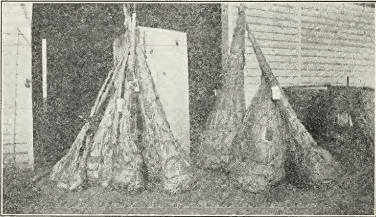
Showing Manner of Preparing Packages for Shipment, Bundles Are First Burlaped, Then Completely Wrapped With Heavy, Tough Paper, Making the Package Practically Frostproof.
