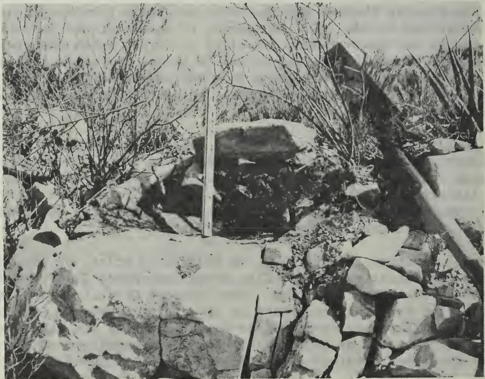
Soil profile, typical of the steeper areas of the watershed (5 inches of stony clay loam over fractured limestone bedrock).
