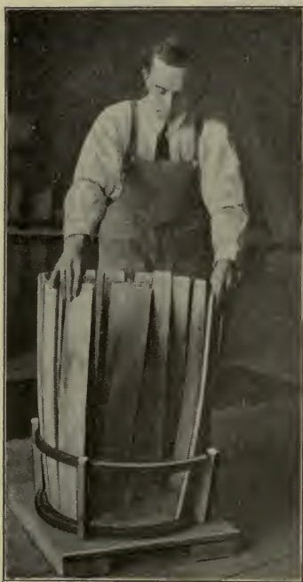
Fig. 38.—FORM FOR SETTING UP A BARREL
