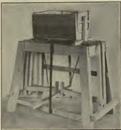
Fig. 71.—A HOME-MADE BOX NAILING PRESS
