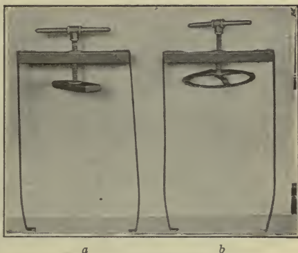
Fig. 50.—TWO TYPES OF BARREL PRESSES b is preferable, as it exerts a more even pressure on the barrel head.
