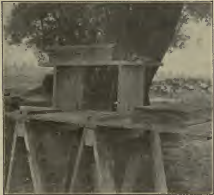
Fig. 33.—A FORM FOR SETTING UP APPLE BOXES
