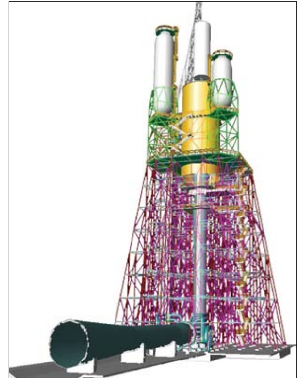
This engineer's concept drawing of the A-3 Test Stand shows the 300-foot-tall structure's open steel frame and large exhaust diffuser.
