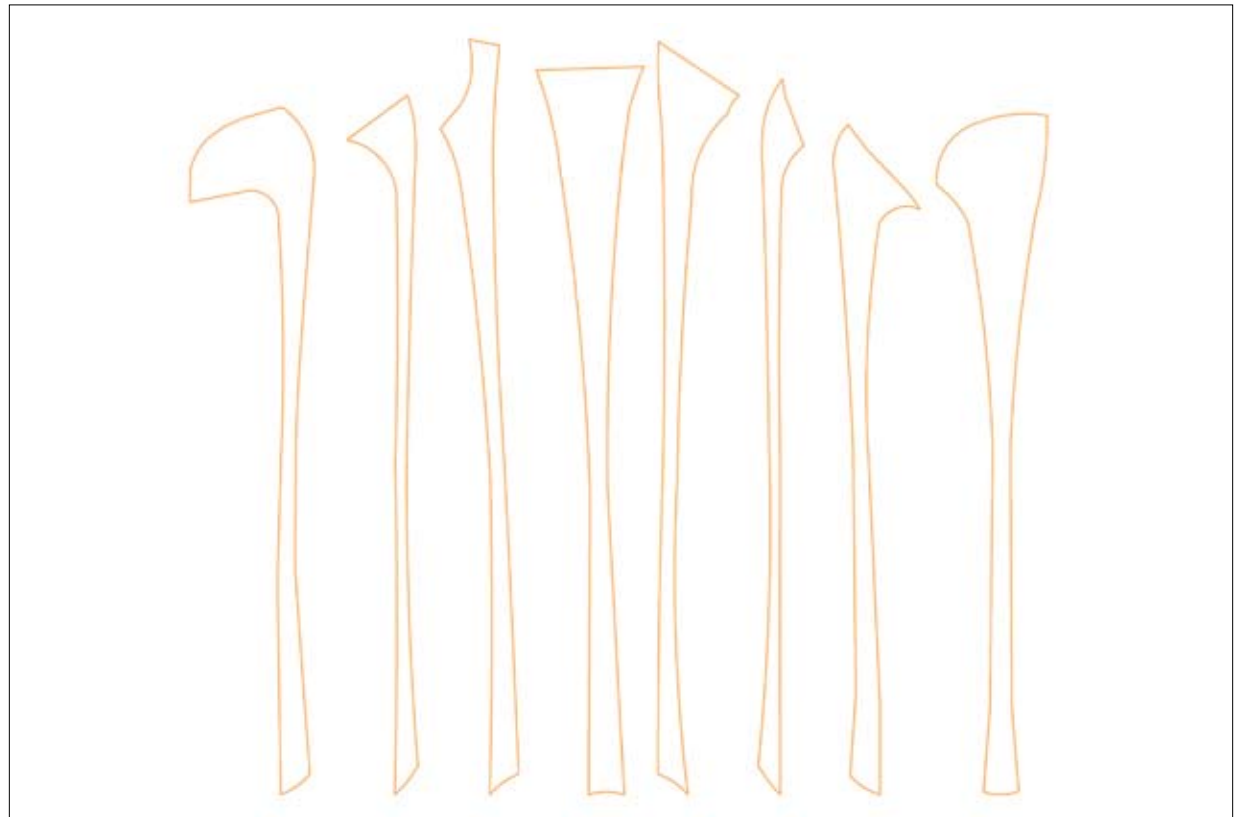
One of the technical challenges faced by the Computational Sciences Group at Glenn Research Center was creating software that was able to accurately flatten a 3-D surface into a 2-D surface.
