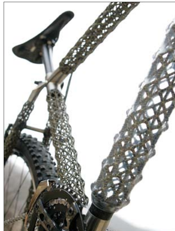
Civil Engineering students at Brigham Young University built an ultra-strong, super-light mountain bike using carbon fiber IsoTrusses instead of regular cylindrical tubes.
