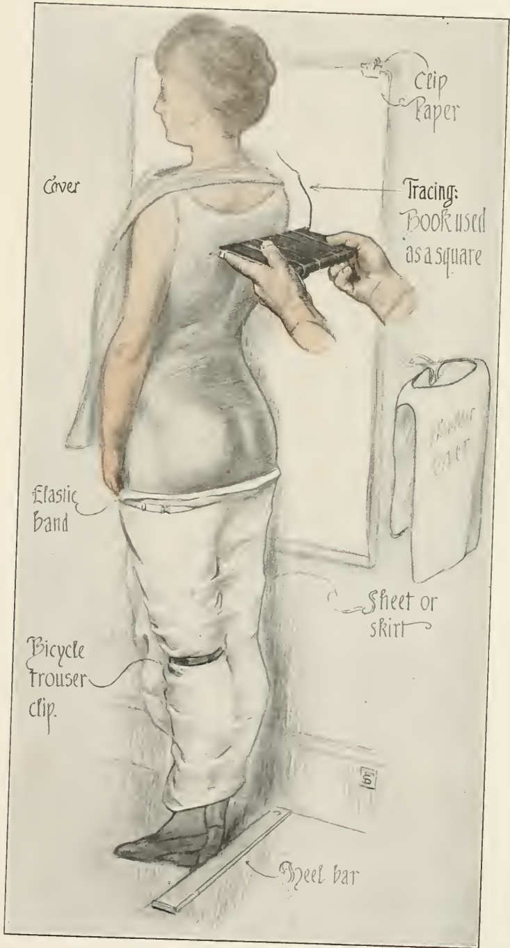
FIG. 35.—Simple method of recording outlines. Against a heel bar the subject stands. The paper is clipped to wall or drawing board. A pencil, held by elastics in the groove of a narrow book that acts as a square, follows the profile and makes a tracing. The knee action is shown by the snug sheet.
