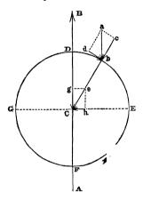
city V - V', that is, with a less velocity than hemisphere D E F; therefore, by axiom D, the pressure of the air on the quadrant D E will be greater than that on the quadrant D G, in proportion to the difference of the squares of their velocities. It is evident then that the force resultant from the whole of the pressure on the hemisphere G D E, must be represented by a line the
