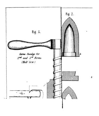
the shell passed through a swedge, in which a steel matrix of the exact size of the shell is cut. The portion of the lead on the slot piece, which in casting had been left beyond the true form of the perfect shell (b b, figs. 1, 2, and 3), is thus compressed round the neck of the tenon, and a perfect waterproof "dovetail" joint is the result. So perfect is this joint, that, when the shell is exploded, fragments of both parts sometimes fly off together, the joint between them remaining unopened.
