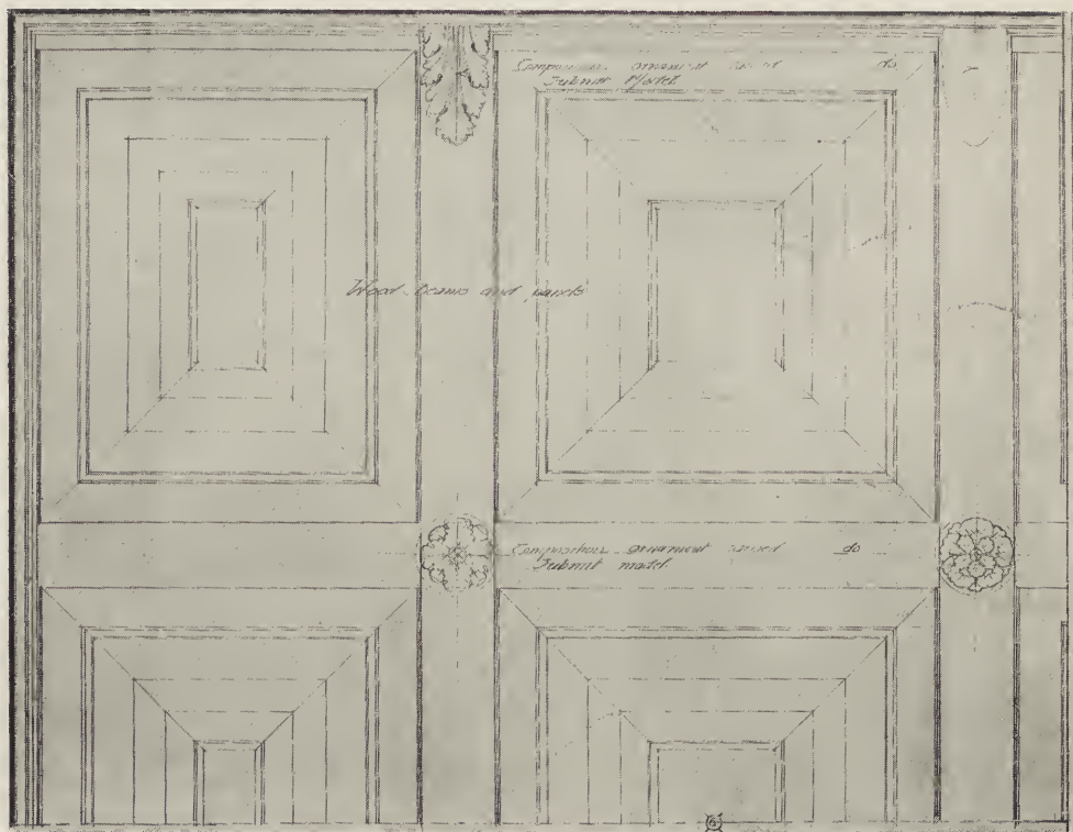
DETAIL OF RECEPTION ROOM CEILING—COUNTRY HOUSE OF H. H. ROGERS, ESQ., SOUTHAMPTON, L. I. Walker & Gillette, Architects.
