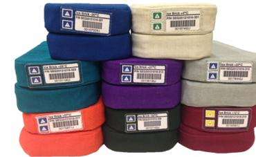
to maintain specific temperatures between -32°C and +37°C. Ice Bricks are reconditioned using active hardware (MELFI, Glacier, Polar, MERLIN).
