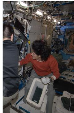
Double Coldbags (DCBs) have highly insulated walls, and are designed to carry payload science at controlled temperatures by utilizing Phase Change Material (PCM) to maintain specific temperatures for a prolonged period of time. The DCB is rectangular and fits in a single mid-deck locker. It is commonly used to transport science to and from the ISS on visiting vehicles.
