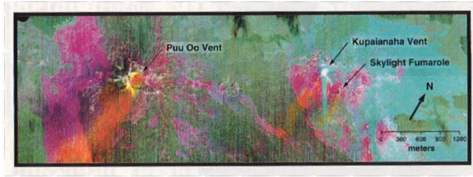
Figure 22. Decorrelation Stretch Applied To TIMS Image Data (Realmuto et al., Figure 2, p. 15060)
