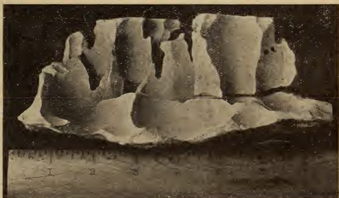
FIGS. 2 and 3. Dolomite from deep water in Georgian Bay, showing solution cavities. Two views of the same specimen.
