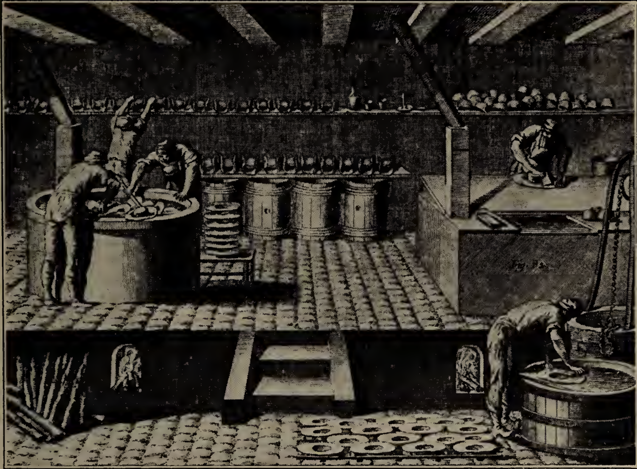
The dye room of a hat factory, 1780. Also carding and shaping brims in boiling water.
