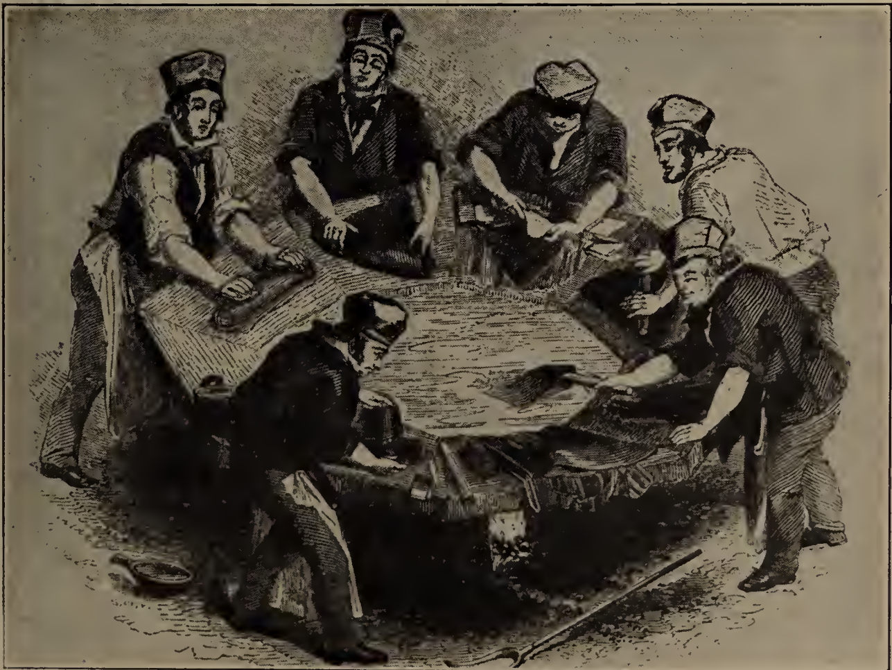
The sizing "battery" in the time of William Connett, 1815.
