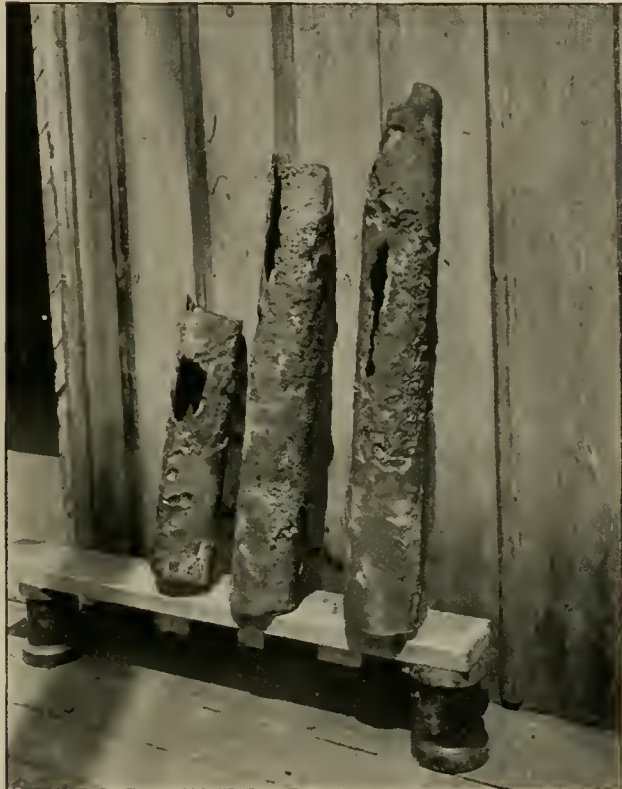
ELECTROLYTIC ACTION AT MILWAUKEE—IRON WATER MAINS.
