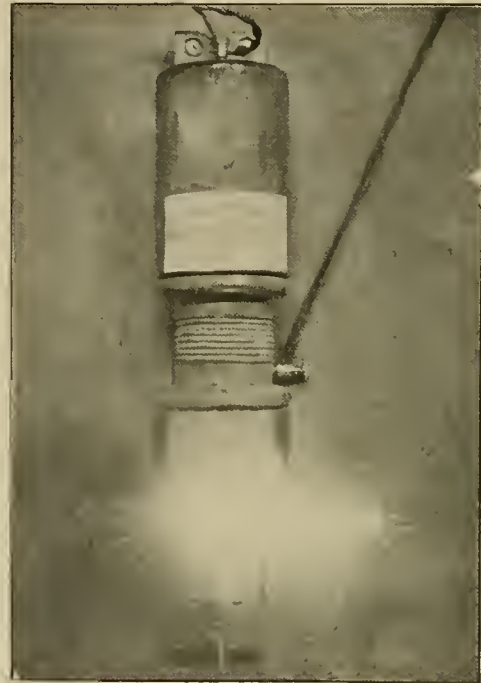
GARTON ARRESTER AT THE INSTANT OF DISCHARGE.
