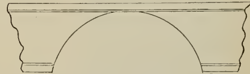
SIDE VIEW OF I BEAM. As cut away for carrying pulley at Gregory Avenue Crossing.
