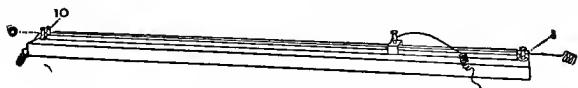
Fig. 5. The rheocord. A metre rule is screwed to the lid of a shallow box of oak. At each end is a binding post. To the post marked 0 is fastened one end of an unbroken German silver wire (No. 30) ten metres in length. This wire passes over the metre stick to post 1, and thence into the box, where the remaining nine metres go to and fro between two rows of pegs at the ends of the under side of the cover of the box. The end of the 10 metre wire is brought out of the box and fastened to post 10.
