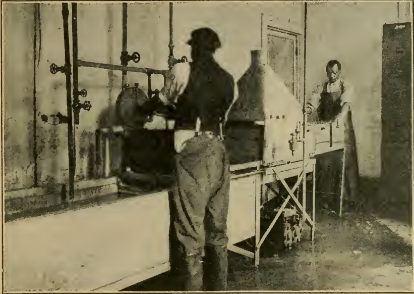
FIG. 19.—Turbine-brush bottle washer. Bottles are rinsed by sprays of boiling water forced into them by pump.
