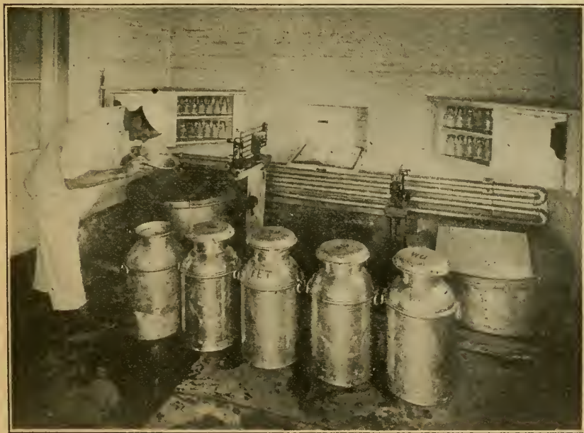
FIG. 1.—Dump or weigh can with platform scales. Tank sunk in floor to make dumping of milk easier.
