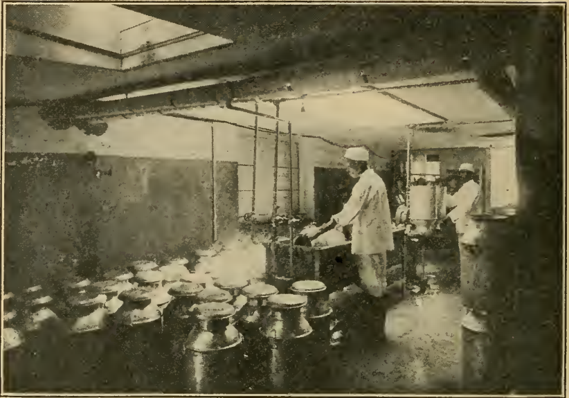
FIG. 21.—Washing, steaming, and drying cans.
