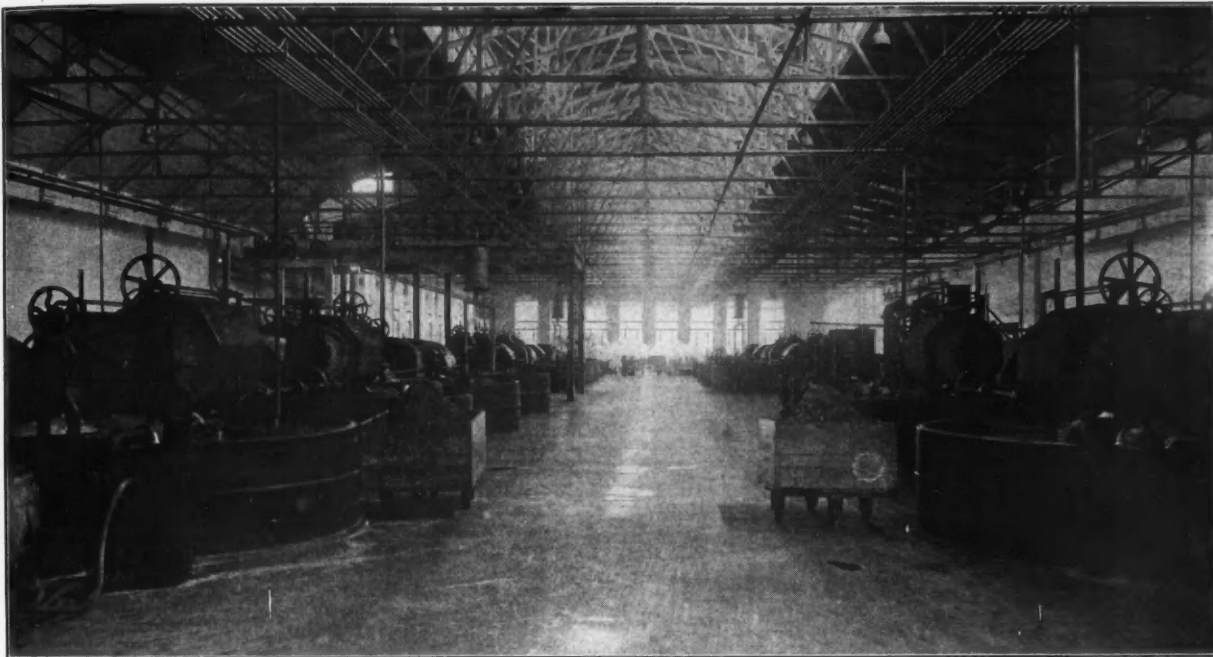
KALAMAZOO VEGETABLE PARCHMENT CO.'S MACHINE ROOM—FOURTEEN 1,000-LB. "HORNE" BEATERS
