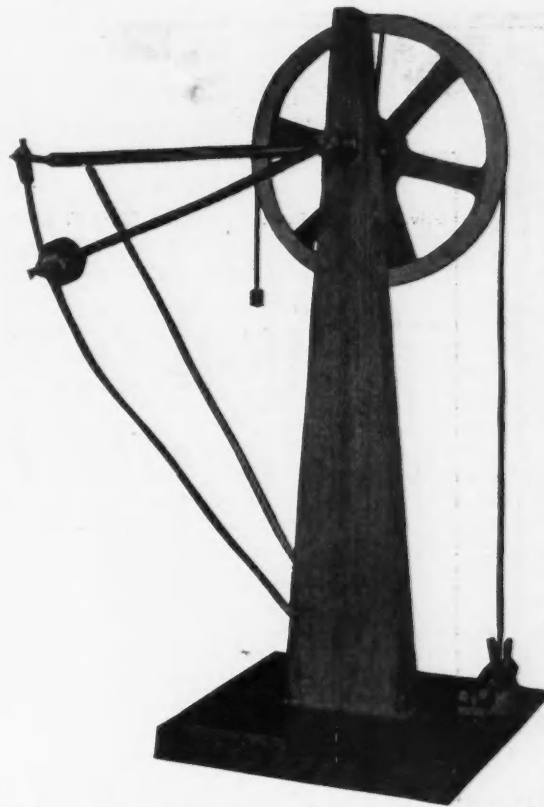
FIG. 1. MACHINE FOR TESTING TEARING STRENGTH OF PAPER
