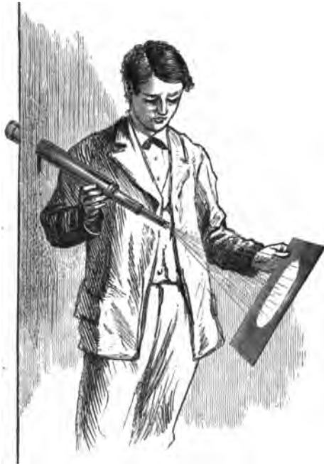
FIG. 65. — Method of holding telescope, to show sun on screen.
