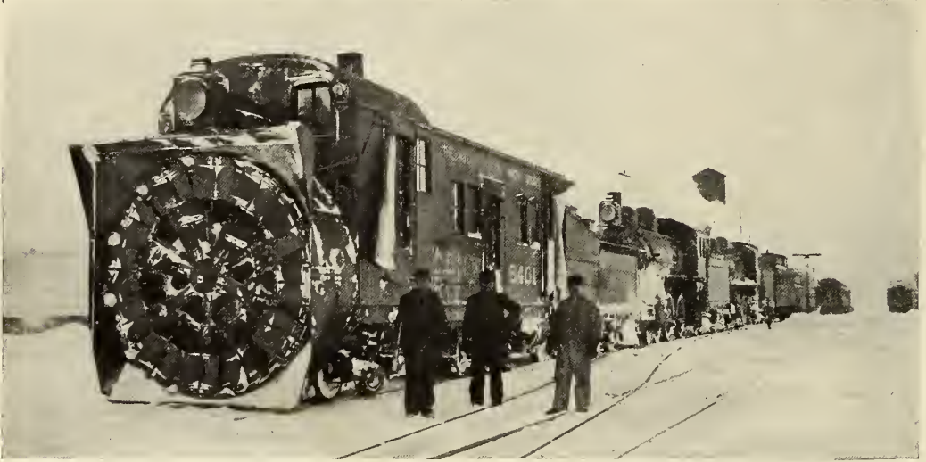
A SNOW-PLOW TRAIN. THE PLOW AND ITS TENDER, TWO ENGINES, AND A CABOOSE.
