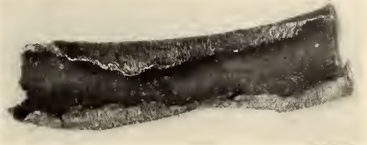
THE LEAD PIPE GNAWED BY RATS.
