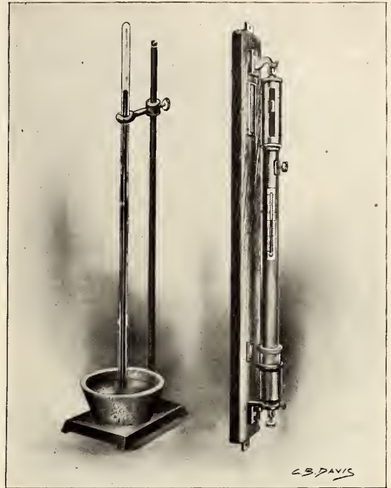
Original type of barometer, mercury in a glass tube.
