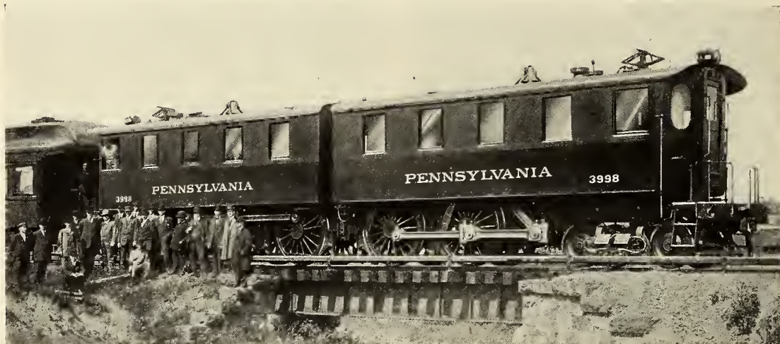
AN ELECTRIC LOCOMOTIVE ON THE PENNSYLVANIA RAILROAD THAT DRAWS THE TRAINS THROUGH THE TUNNEL UNDER THE HUDSON RIVER.
