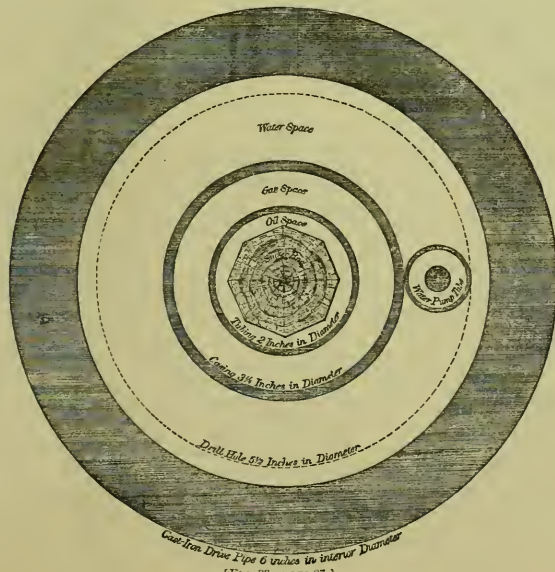
Cross-section of pumping well, 1868—cast-iron drive-pipe.
