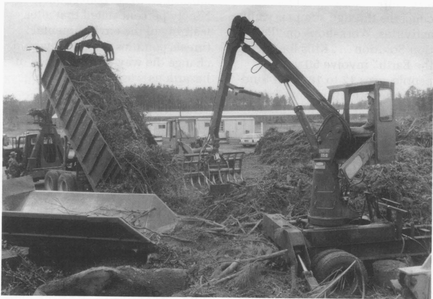
Mountains of yard trash are converted into compost, mulch, fuel wood, and landscape chips at Wood Resource Recovery, Inc., in Gainesville, FL. The composting demonstration project shows the feasibility of composting yard trash from a typical municipal solid waste stream.
