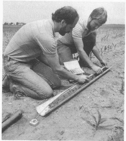
Neil Eash and Aaron Steinwand, ARS research associates, examine a soil core sample. Samples will be analyzed to see how nitrates and other nutrients are distributed, and to locate carbon accumulations from decaying organic matter. Lowell Georgia/USDA 89BW1229-10
