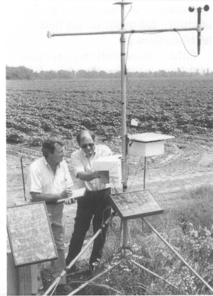
Electronics Engineer James McKinnon (right) and Frank Mitchner, a Mississippi cotton farmer, review information from an automated weather station. The station feeds daily weather information into Mitchner's farm computer to update predictions for cotton yield and harvest dates. Tim McCabe/USDA 0786X0791-28
