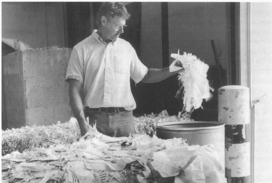
Bob Kelley, physical science technician at USDA's Forest Products Laboratory in Madison, WI, takes samples of laser- and photo-copy waste paper from bales of mixed office waste. The samples are used in recycling research aimed at de-inking difficult-to-recycle waste papers.
