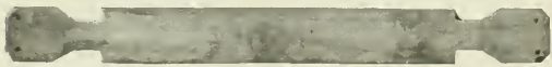
Steel Plate After Having the Ends Shaped and the Rivet Holes Punched.
