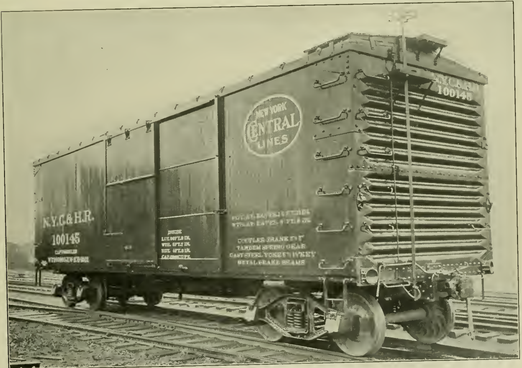
Steel End Applied to 40-Ton Wooden Box Car; New York Central & Hudson River.
