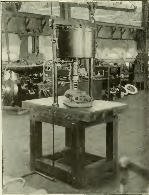
Fig. 14—Pneumatic Press for Bushing Work.
