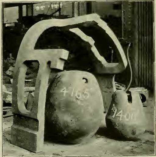
Vanadium Cast Steel Locomotive Frame After Drop Test.
