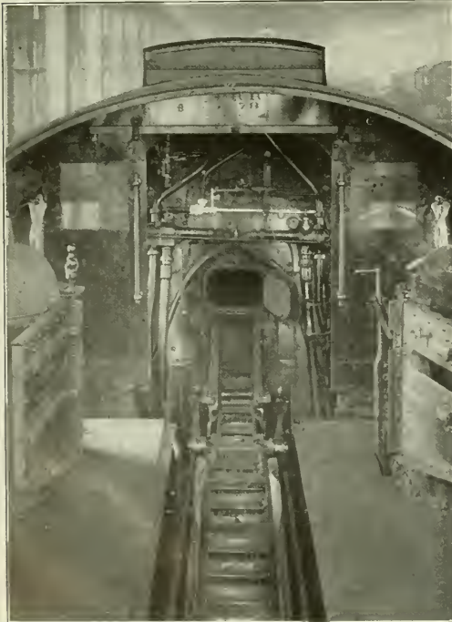
Arrangement of the Coal Conveyor on the Gee Stoker.
