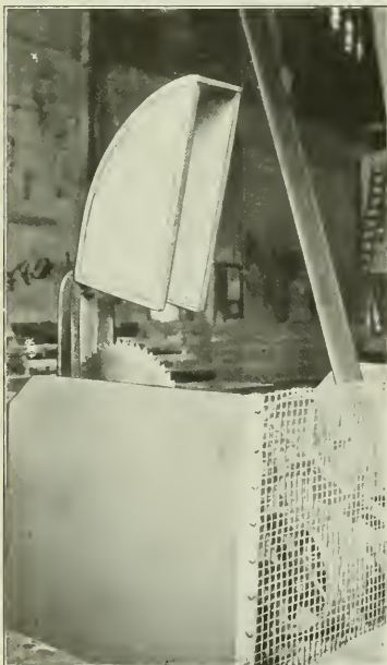
Fig. 14—Guard on Swing Rip Saw in Open Position.
