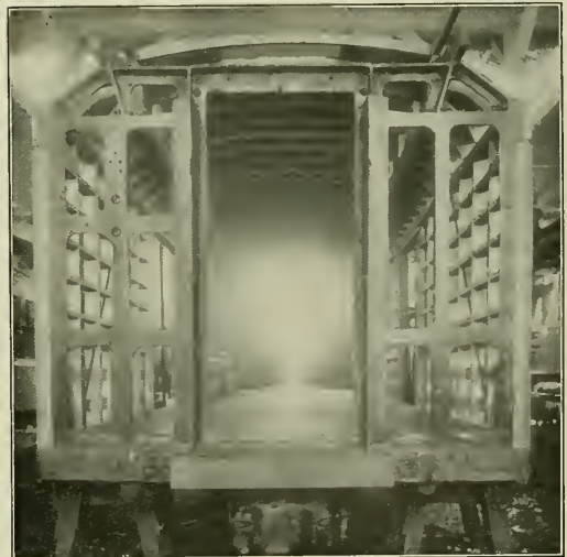
Cast Steel End Frame of Baggage Car.
