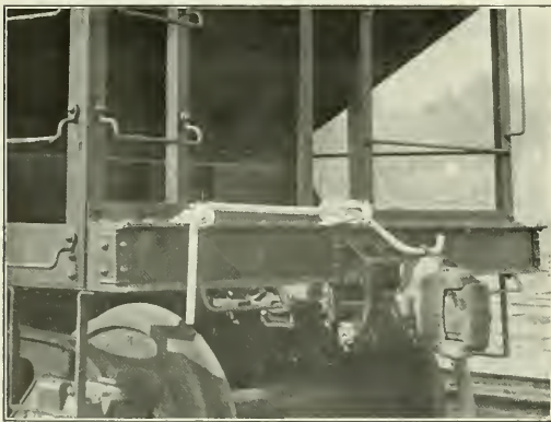
Coupler Release Rigging on a Hopper Car.
