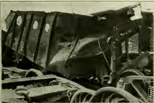
Fig. 3—Hopper Car Damaged in a Wreck.
