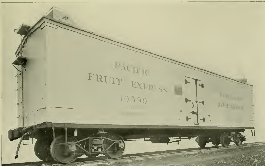
Refrigerator Car with Bettendorf Steel Underframe.
