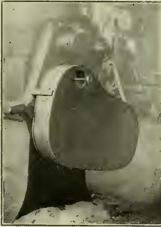
Fig. 17—Guard for Lathe Feed Gears.
