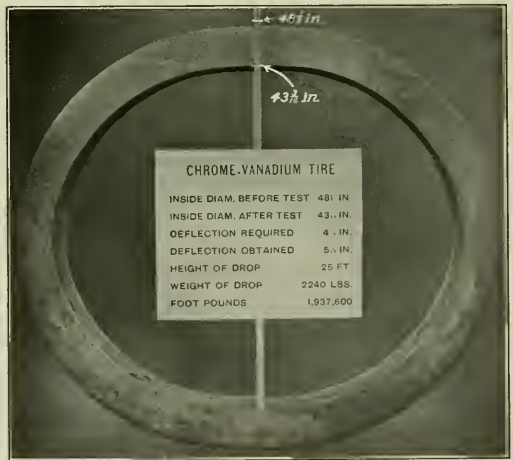
Chrome-Vanadium Driving Tire After a Drop Test.
