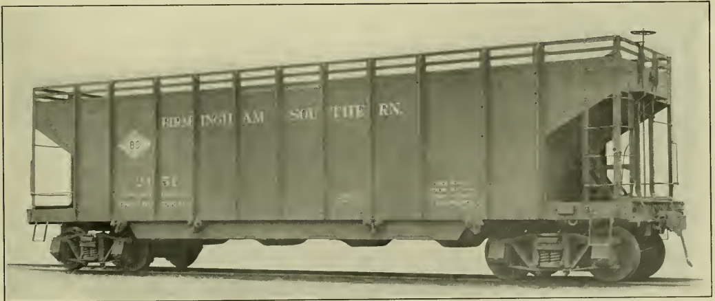
Seventy-Ton Capacity Car with Four Hoppers.
