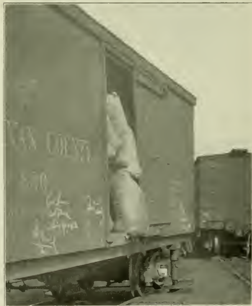
The Effect of a Lack of Doorway Protection on a Shipment of Feed in Bags.
