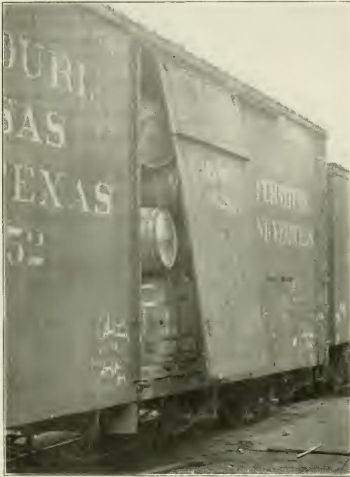
Door Burst Open by the Shifting of a Shipment of Barrels.
