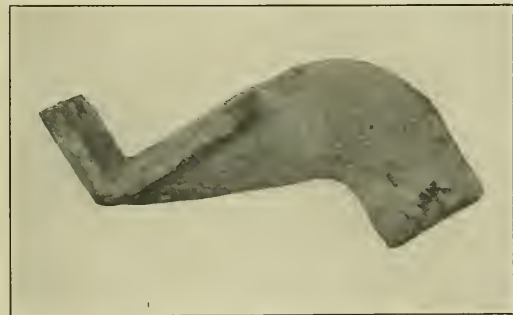
Transom End After the Parts Are Welded.
