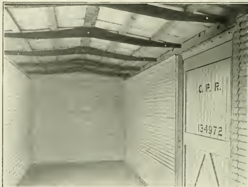
Interior of Canadian Pacific Corrugated Metal Sheathed Box Car.
