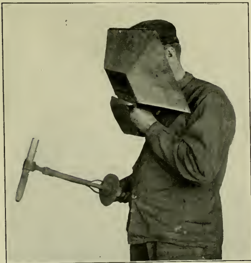
Graphite Electrode Holder and Hand Shield.
