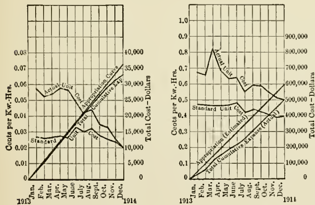
FIG. 3.—VISUALIZED RECORDS OF THE ENTIRE COST OF POWER PLANT OPERATION, IN WHICH THE ACTUAL UNIT COST AND THE STANDARD UNIT COST ARE PLOTTED TO THE SAME SCALE.
