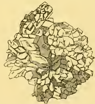
FIG. 19.—Basalt of Christmas Harbour. Grouped granules of olivine, imitating the form of this mineral in the chondres of meteorites. \frac{1}{2} crossed nicols.
