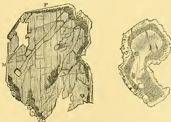
FIG. 11.—Andesite of Ascension. Sections of plagioclase corroded by the magma, with a zone of small scales of hematite; the external felspathic zone is labradorite, the internal part of the plagioclase is more acid, the extinctions of which are those of andesine. \frac{2}{5} crossed nicols.
