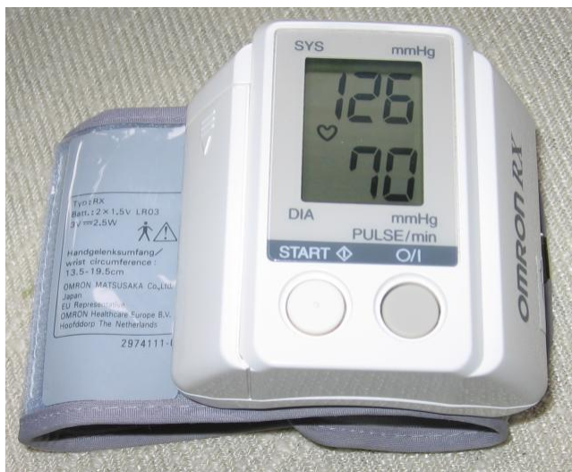
Figure 1: A digital sphygmomanometer is made of an inflatable cuff and a pressure meter to measure blood pressure.
