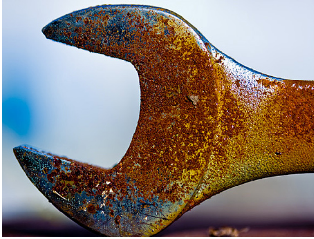
Figure 3: Rust is the result of a chemical reaction between iron and oxygen.
