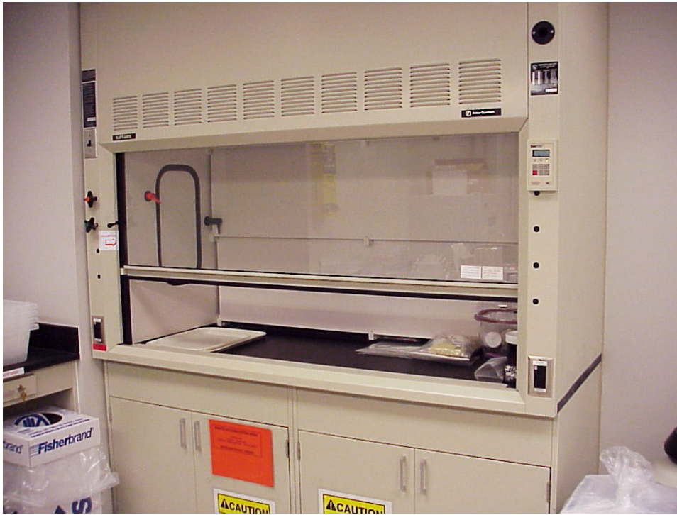
Figure 8: A laboratory fume hood. This laboratory hood sucks dangerous fumes out of a lab and allows researchers to work with dangerous chemicals without breathing them.
