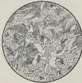
FIG. 6. Ophitic texture of normally crystallized basalt. (Slide No. 47.) Plagioclase laths, diopside granules, and crystals and dust of magnetite in mutual intergrowth. The magnetite is mostly included in the diopside, but partly also in the plagioclase. Diameter of field 1\cdot 5^{\text{mm}} .
