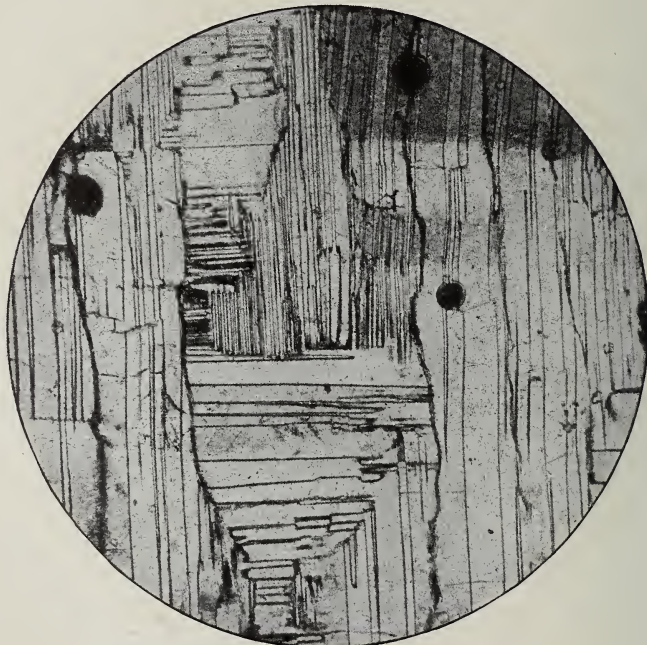
FIG. 1. Polysynthetic albite-like twinning on artificial soda anorthite. Nicols crossed. Magnification 85 diameters.
