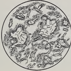
FIG. 1. Typical structure of the vitrophyric phase resulting from quick chill. (Slide No. 105.) Elongated crystals plagioclase, stouter forms diopside, matrix light-green glass, perfectly isotropic. Actual diameter of field 1.5 mm .
