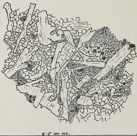
FIG. 8. Modification of forms of plagioclase and diopside resulting from simultaneous crystallization. A few magnetite grains (black) and some chlorite (gray) are also present (Slide No. 64).
