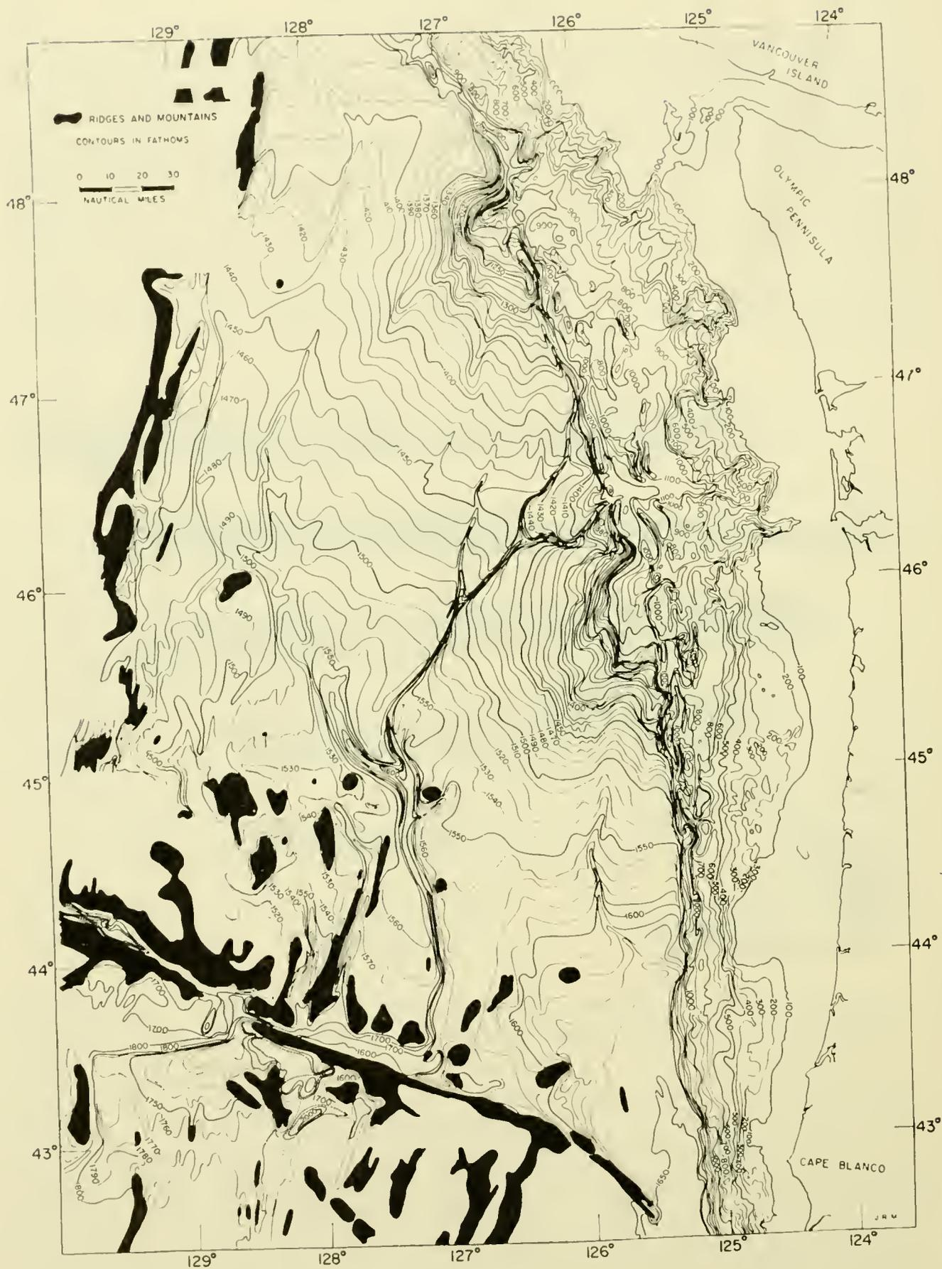
Fig. 27. Caseadia Canyon and Interplain Channel. Note how the tectonic trough between 43° and 44° North has acted as an abyssal gap. The Caseadia Submarine Canyon, which has apparently built the large cone shown in the northern part of the chart, passes through this abyssal gap and has supplied sediment to the abyssal plains lying to the west of the area shown on this map. (After Hurley, 1960.)
