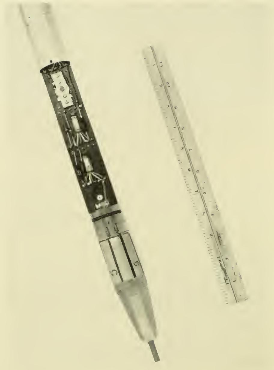
Fig. 2. The barium titanate pressure-sensitive element and part of the preamplifier of the hydrophone used below sono-radio buoys. Scale in inches.
