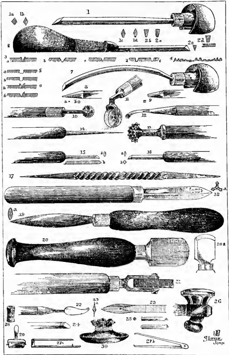
FIG. 1.—The Tools used in the various Methods of Engraving and Etching.
