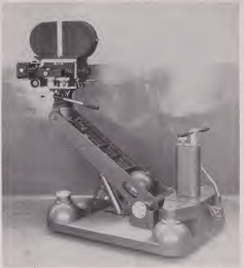
FIG. 1—Low-slung chassis is just one of many features of the Multidolly, newest baby mobile mount for film and TV cameras. Other features are differential circular steering and hydraulic boom control.
