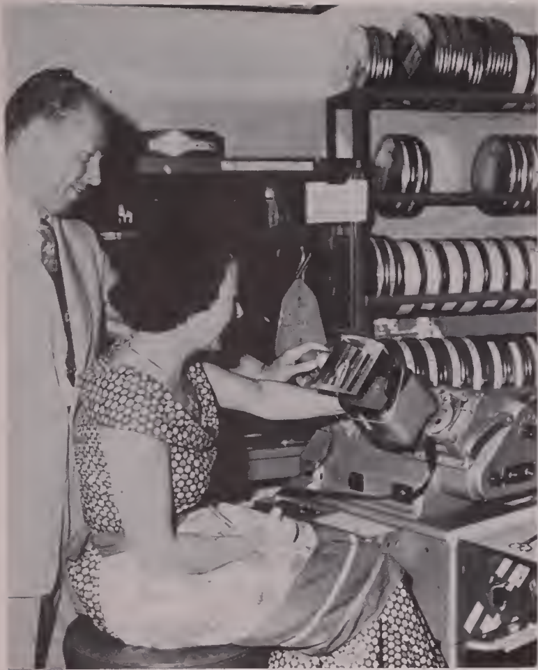
TO EDIT CinemaScope films, it became necessary to devise a special auxiliary Lucite lens for Moviolas, which transforms the squeezed image on CinemaScope films to full panoramic width. Examining the new viewing attachment is TCF Cutting Dept. head Jerry Webb and film editor Barbara McLean.
