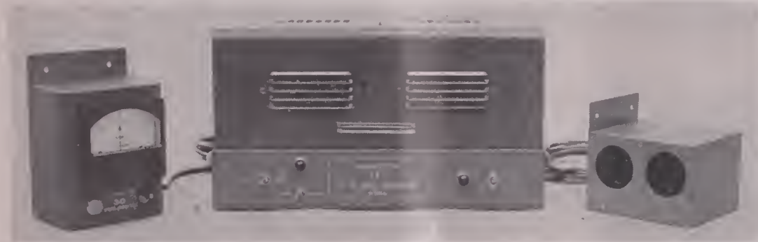
FIG. 5—Polaroid 3-D Electronic Sync Monitor, model 21, which automatically indicates any out-of-sync condition in 3-D projection of \frac{1}{4} frame or more and enables projectionist to correct it. When theatres are thus equipped, comfortable viewing of 3-D films can be assured.
