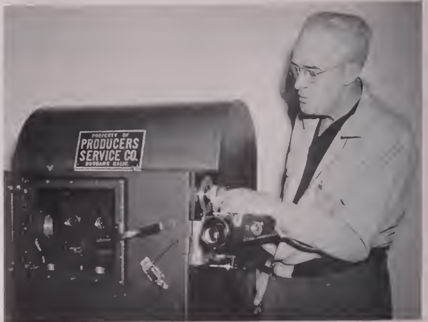
FULLY BLIMPED camera, showing external controls for focus, and the Mitchell-type finder. Beside camera is cinematographer-technician Gordon Pollock, ASC, who collaborated in designing the camera.
