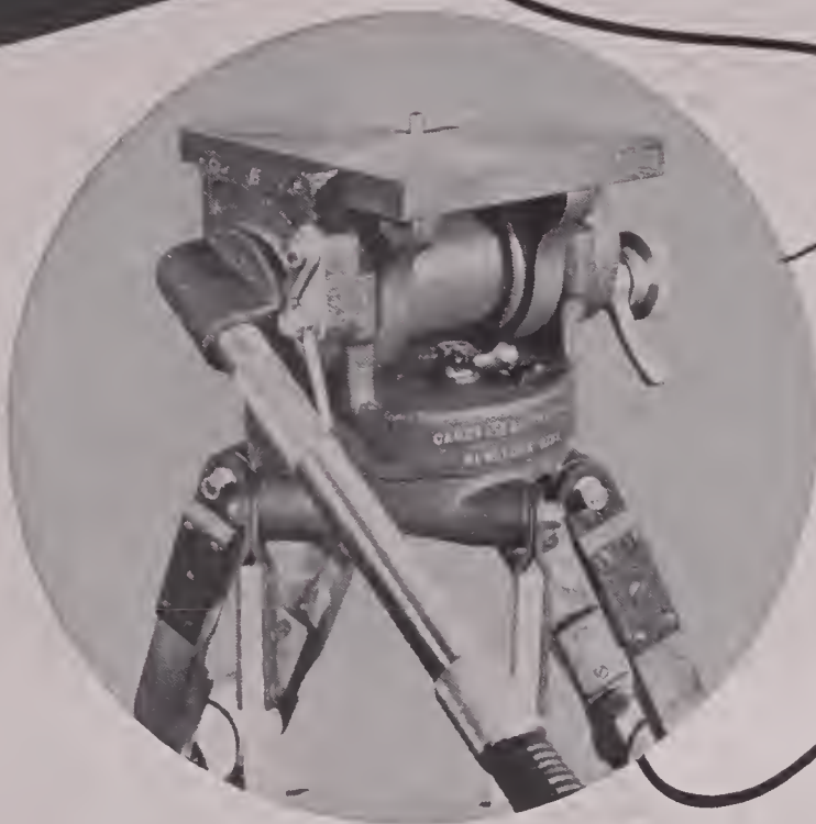
HEAD ILLUSTRATED CONTAINS ADJUSTABLE CAMERA TIE-DOWN SCREW FOR LOCATING CENTER OF GRAVITY. THIS FEATURE IS OPTIONAL.
