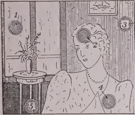
FIG. 1—Image as seen in camera finder system, at point 15 in Fig. 3 at right. The photo-cell on prober (Fig. 2) is moved over area to make readings at 1, 2, 3, 4, and 5.
