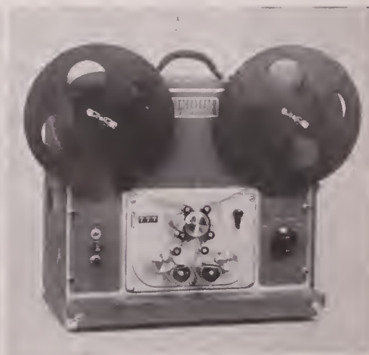
FIG. 3—Portable rack-mount version of the Magnasync recorder. Clutch overdrives and separate motors control takeup, rewind.
