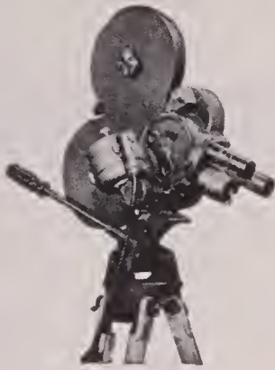
PERFECT PERFORMER. 16mm 70-H camera. Seven film speeds, governor controlled—three-lens turret with positive-type viewfinder system—shutter stabilizer—hand crank, rewind knob—adapted for external magazine and electric motor.
