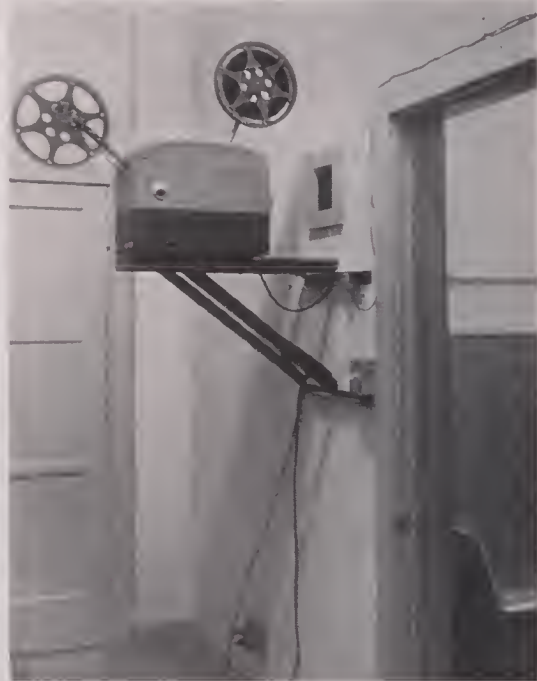
METHOD of mounting 16mm sound projector in adjoining room, which serves as projection booth. No gloss is used in the port.
