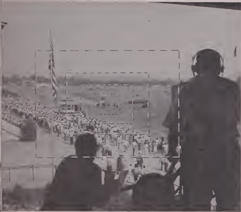
DOTTED LINES show picture area taken in by the Pan Cinor in a typical zoom shot of a horse race—recording the scene in a range from 20mm focal length down to 60mm.
