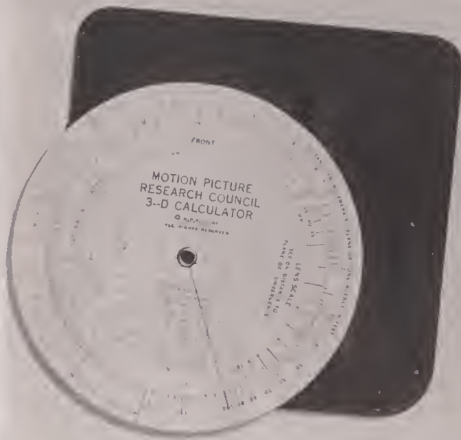
THE MOTION PICTURE Research Council 3-D calculator, which enables a cameraman or his assistant to rapidly determine proper camera settings to achieve the perspective and stereoscopic depth necessary to acceptable 3-D cinematography.
