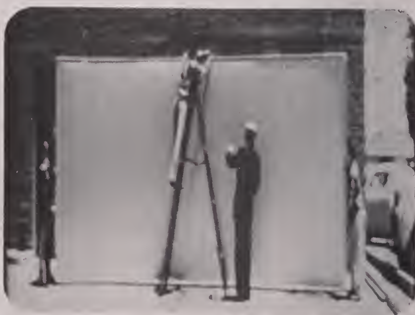
for Vistarama presentation. Distortion of image is result of "squeeze" action of the Vistarama lens. Image is expanded in projection and appears normal on wide screen having aspect ratio of 2.66 to 1.
