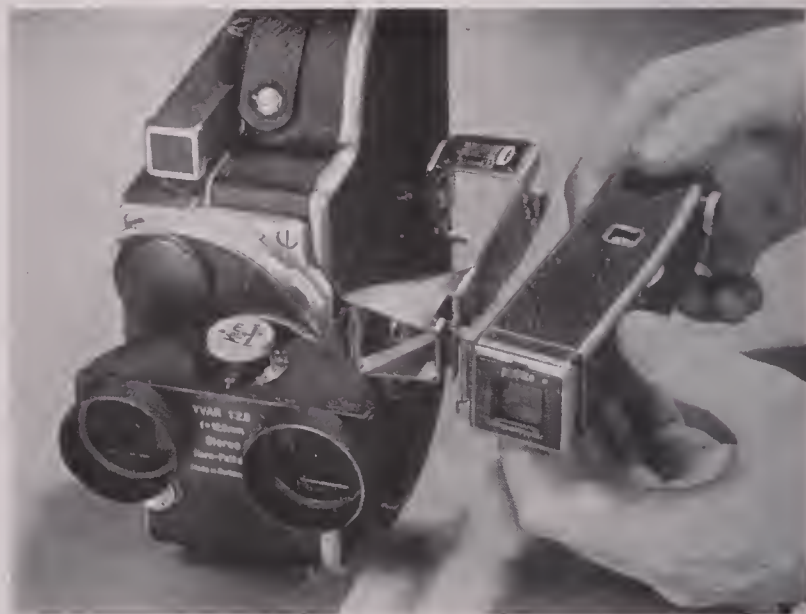
FIG. 2—The Bolex Stereo taking lens may be used only with the Bolex DeLuxe H-16 camera. Here the stereo mask has been clipped to front of the Octometer finder, which is then attached to the offset bracket for filming 3-D movies.
