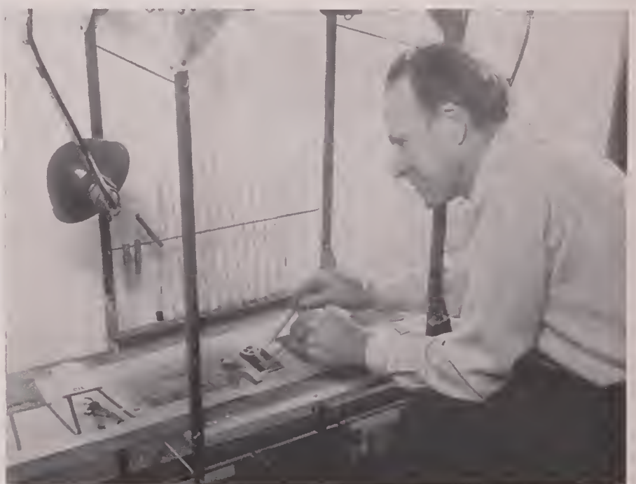
INTRICATE MOVEMENT OF the parts of figures (arms, legs, etc.) is effected through use of long, sharp pins, which gives more precise positioning of parts than if moved by hand. Here also are shown the positioning guides—vertical wires at rear.
