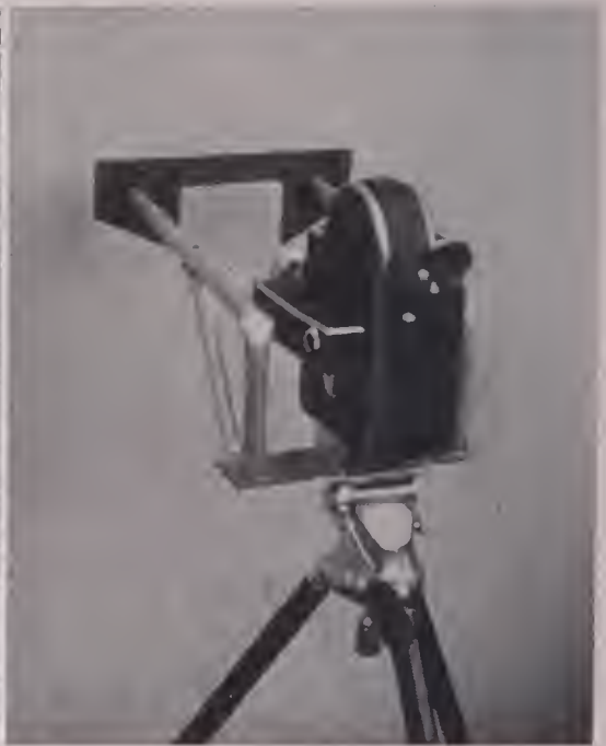
FIG. 3—For extreme closeups, a focal frame will insure sharp focus and center.
