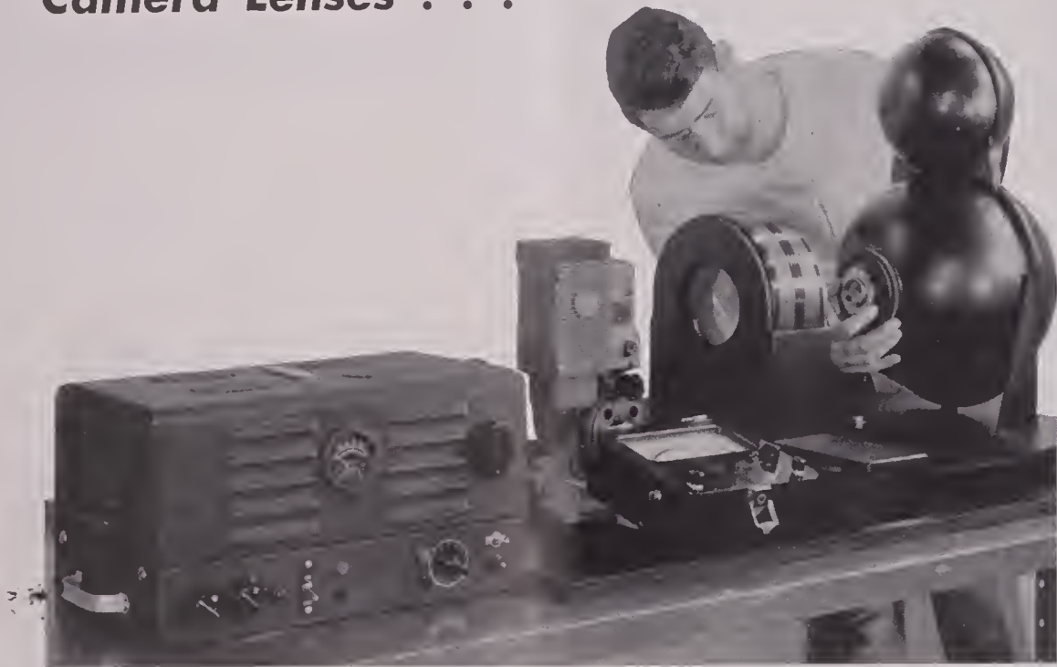
PRC has the most modern scientific equipment for the accurate measurement and calibration of the light transmission of lenses.
