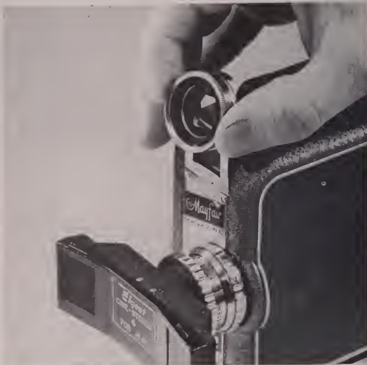
VIEWFINDER unit slips over front element of camera finder, thus adapting it to stereo filming. Here, also, the Elgeet 3-D attachment is shown mounted in place of regular lens.
