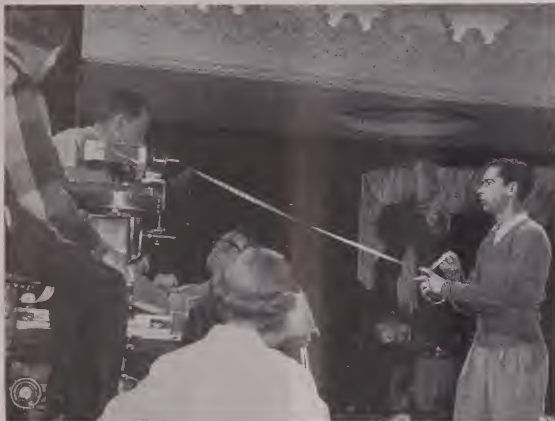
FIG. 1—The "Lazy-8" camera being lined up for a shot for Paramount's "White Christmas." Here may be seen the horizontal position of camera with film magazines on side and the viewfinder on top of the camera. On normal sound takes, a blimp is used.
