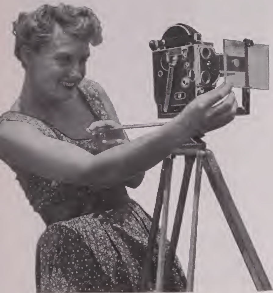
FIG. 1—To prevent thrown objects from damaging the Bolex stereo lens when filming extreme 3-D effects, the author mounted a panel of shatter-proof glass before the lens, as shown above.
