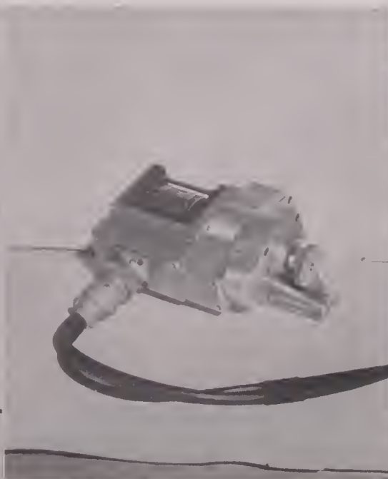
FIG. 3—Motor unit which couples to the camera and actuates the lens control knob. When mounted, it appears as shown above in Fig. 1.
