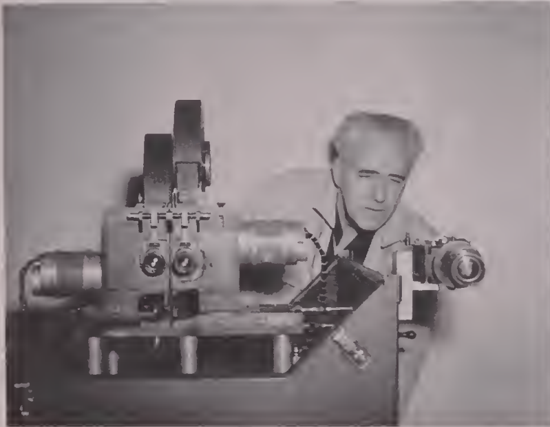
RANGE of camera's interaxial is illustrated in photos above and at right. Interaxial is changed by moving cameras laterally. Here cameras are shown at minimum position, giving an interaxial of 1.9 inches.
