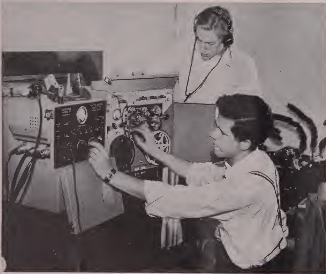
YOU'LL PROBABLY choose one of the popular magnetic recorders for your first sound production. They're simple to use and provide advantages not found in optical sound systems, chief of which is ability to immediately play back tracks for approval or correction. Here a non-professional group records sound for a college film production in 16mm, using magnetic equipment.
