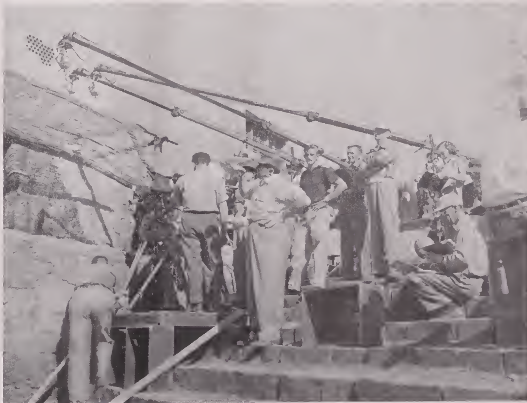
THE "NEW LOOK" behind today's scenes in film production. Three mike booms support microphones above set for recording stereophonic sound for CinemaScope, posing new problems for the director of photography.
