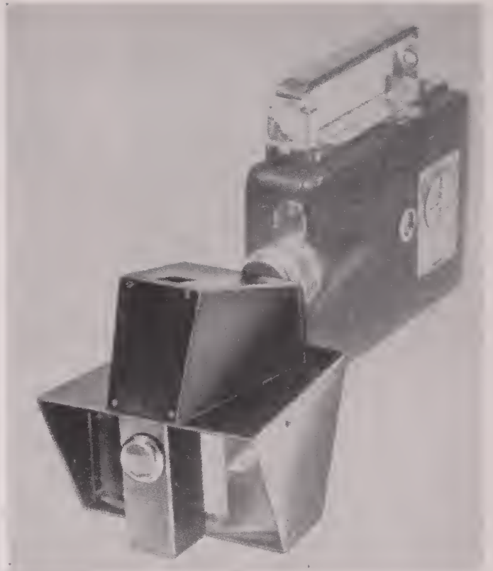
THE NORD STEREO ATTACHMENT for cine photography is called a 'converter.' This is attached to camera by means of bracket fastened to tripod socket. Camera viewfinder is dispensed with, and pictures are lined up through the reflex viewfinder in top of converter.
