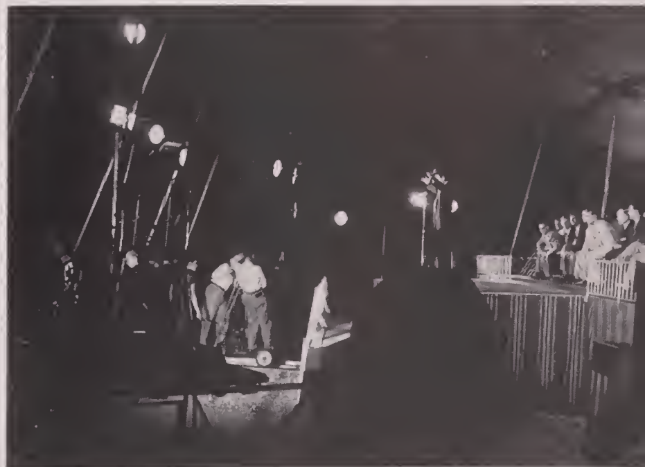
SENIORS AND SKY PANS were mounted high on the central tent poles to give ample light coverage for the many long shots that were made inside the tent on 16mm color film for "Venture Into Faith."
