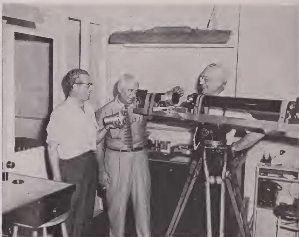
A TELESCOPIC apparatus producing "an artificial star" is used by the studio to test accuracy of new CinemaScope lenses. Above, camera department head Sol Halprin, ASC, checks new lenses, aided by Campbell Forsyth and Grover Laube.
