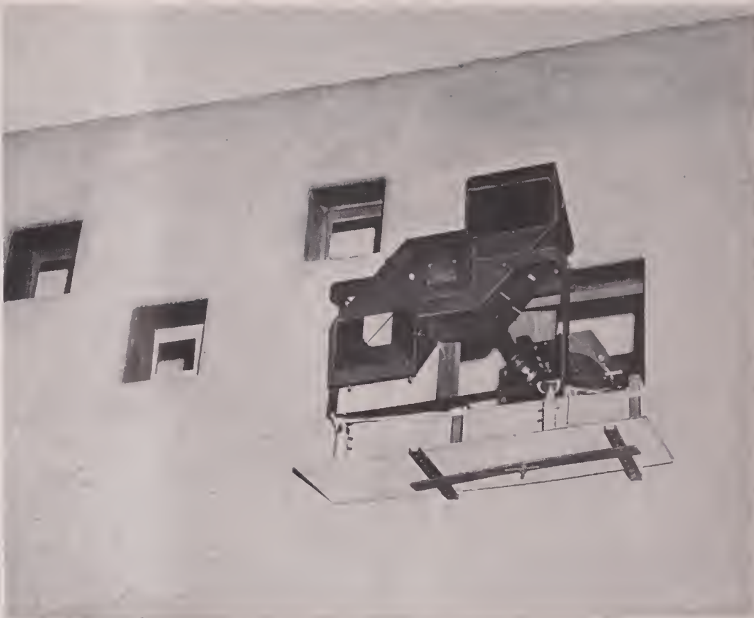
FIG 1—Showing simple installation outside projection booth of the new Nord 3-D single-strip projection system. Units are also available for installation inside the booth. Optical system rotates the twin film images 90° and throws them on theatre screen erect.
