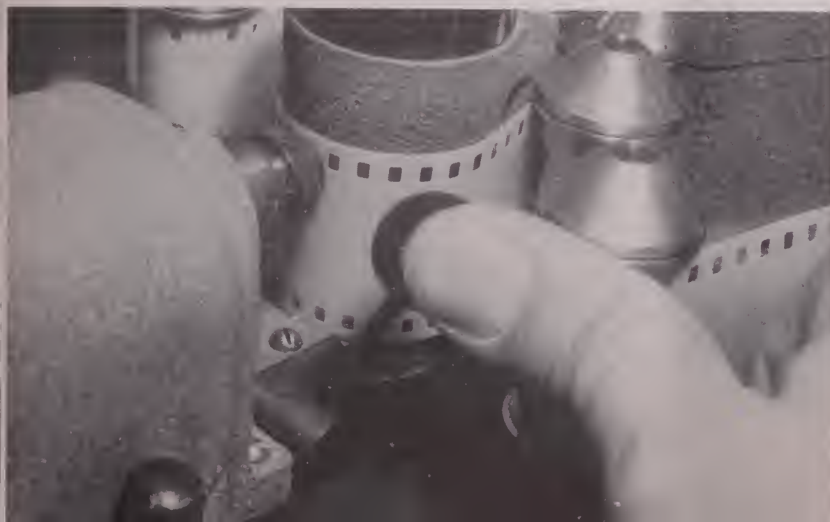
FIG. 6—Film marker at the sound aperture. Pressing lever punches small chip from film which drops into receptacle beneath equipment.
