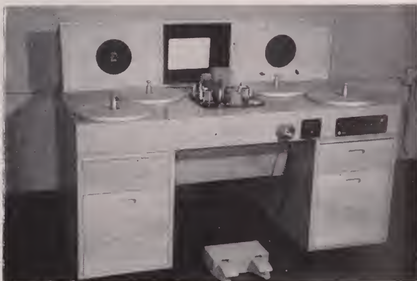
Fig. 2—Foot pedals control forward and reverse motion of films.
