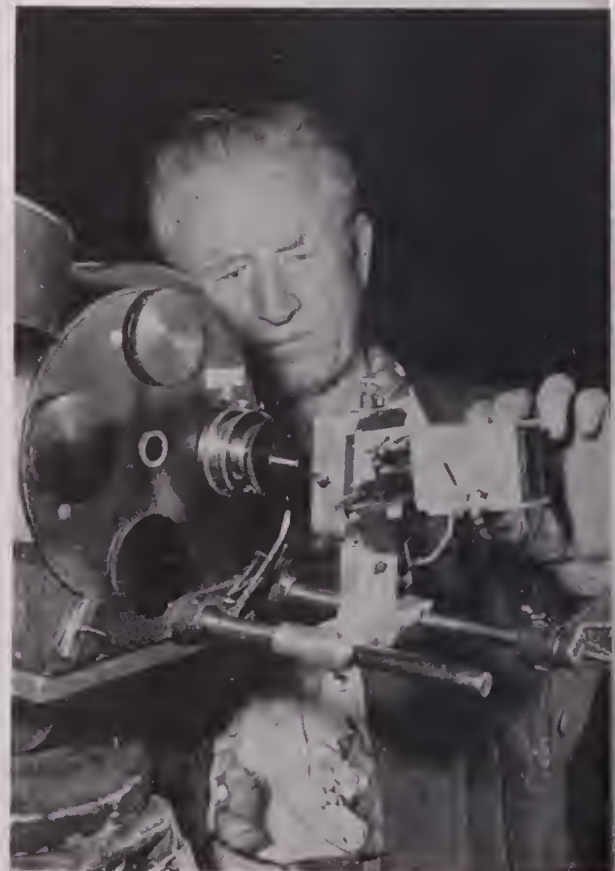
▶ CAMERA assistant Lee Crawford shows how the CinemaScope lens is mounted on camera. Secured in a special mount, lens must be focused in synchrony with camera lens.
