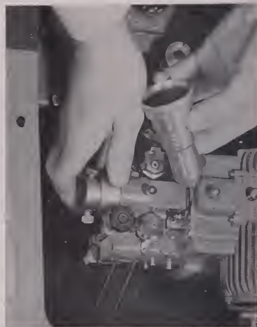
TO PROJECT 3-D movies made with the Bolex camera, a special lens is provided for the projector. The attachment may be used with almost any 16mm sound or silent projector.
