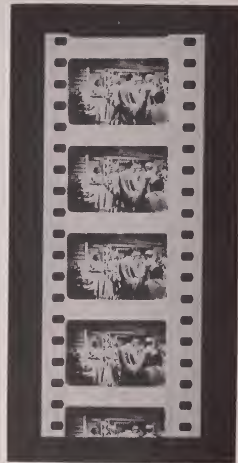
FIG. 5—Full size reproduction of 35mm release print made from the double-frame negative above, left. Latter is optically printed down to area shown, at same time turned 90°. Resultant print gives wide screen picture having greatly improved resolution.
