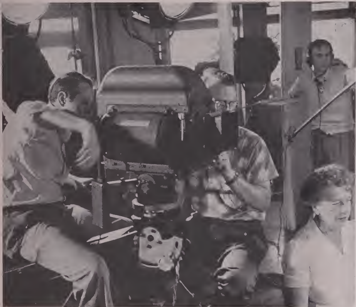
TYPICAL OF the modern cinematographic equipment which the USC students used in filming "Let Me See" is latest Mitchell "16" camera shown here in hands of Richard Harber and Robert Keifer filming a dolly shot on an indoor location.
