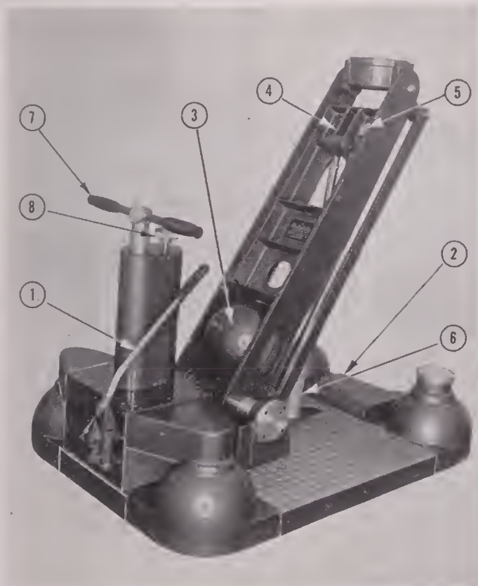
FIG 2—Basic hydraulic circuit of Multidolly: (1) hand pump; (2) fluid reservoir; (3) pressure accumulator; (4) pressure gauge; (5) valve; and (6) cylinder. Boom is lowered by releasing hydraulic pressure from cylinder.
