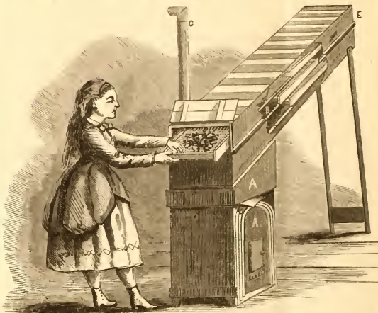
A—STOVE. B—HOT AIR CHAMBER. C—DRYING BOX. D—TRAY CONTAINING FRUIT BEING PLACED IN PROPER POSITION FOR DRYING. E—OPENING FOR REMOVAL OF DRIED FRUIT. F—SMOKE PIPE.
