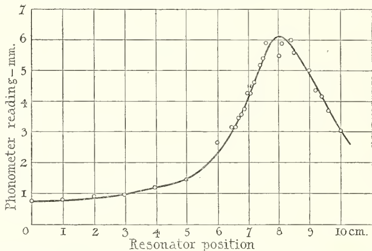
Fig. (ii). Resonance curve of Webster phonometer with reference to sound-waves generated by the diaphone.
