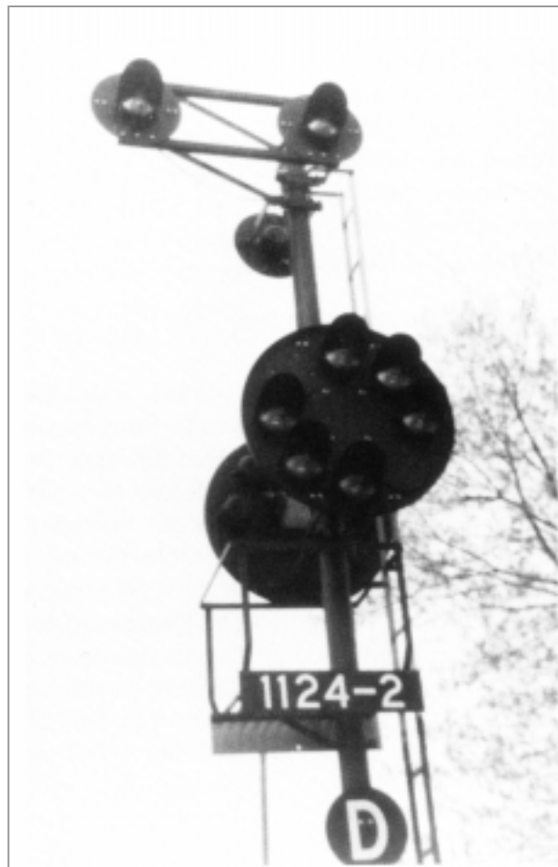
Figure 10--Signal 1124-2. The “D” was added after the accident.
