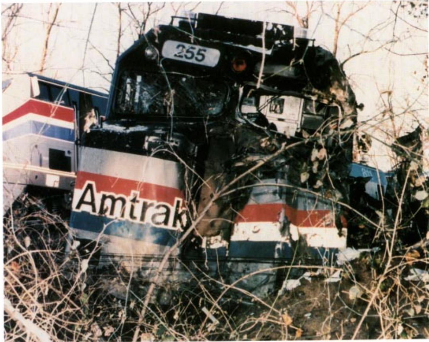
Figure 8--Photograph of postcollision Amtrak locomotive unit ATK 255 at accident site.
