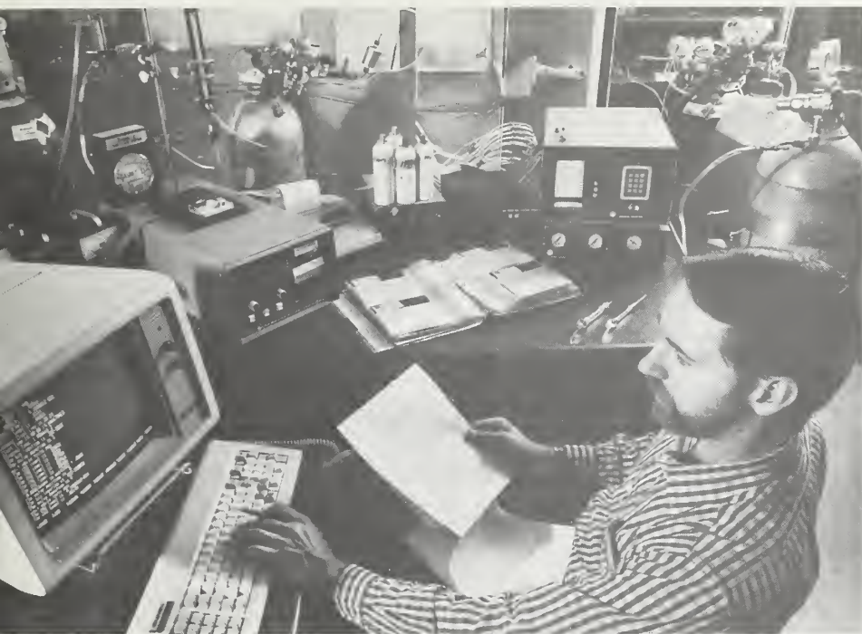
Above: Biochemist Jerry Varns evaluates potato storage environment by computerized monitoring of windspeed, temperature, relative humidity, and gases released by potatoes. (1086X1150-18)
