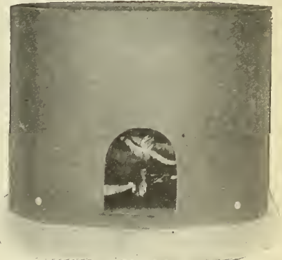
The feather hover inside can be raised and lowered to suit the size of the chicks.
