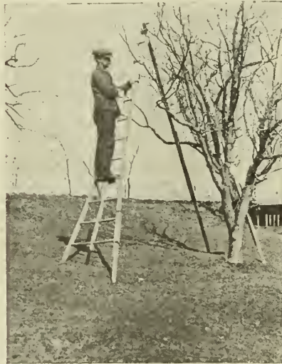
Orchard ladder in use trimming outer branches of a tree. Notice slope of ground, no branches touched by the ladder, which is supported solely by the extended brace standard with no stay chains attached. (See Readers' Open Forum.)
