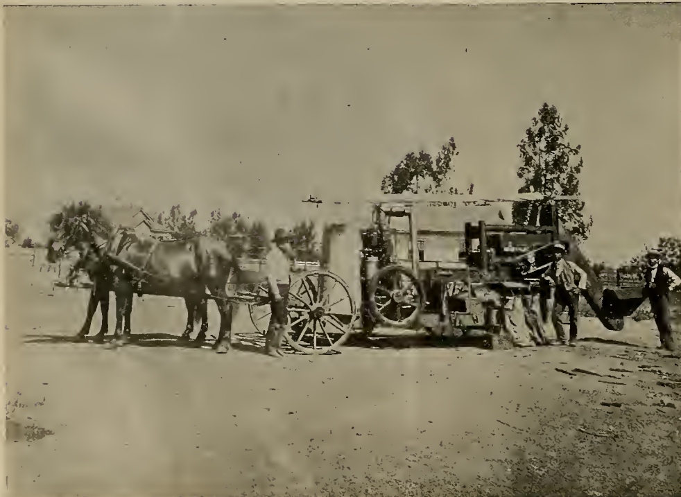
Portable Barley Crusher with 20 H. P. UNION Engine.
