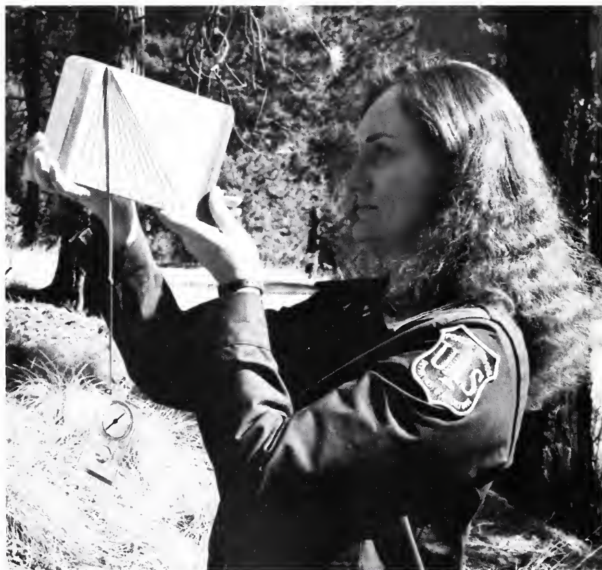
Figure 3 —Sight along the edge of the board parallel to the slope. Read slope to the nearest 5 percent. (Turn the board around to sight downhill.)
