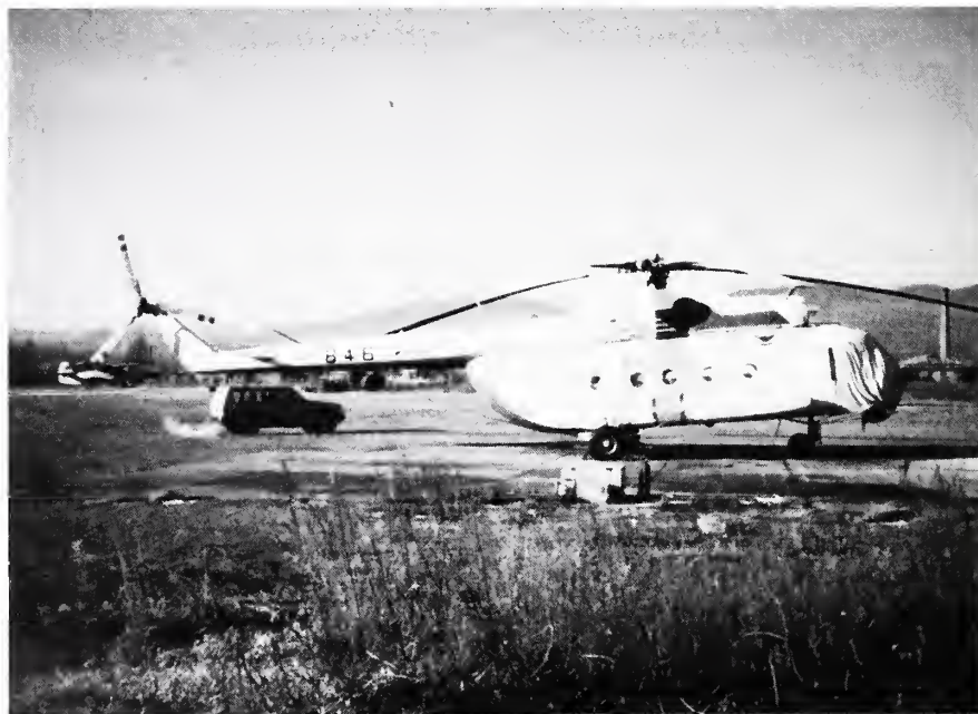
Mi-8 Russian-designed helicopter used by the Chinese for helitack, aerial detection, and transportation of smokejumpers.
