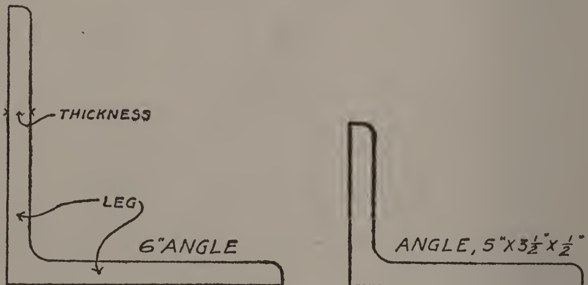
Fig. 140. Steel Angles with Even and Uneven Legs.
