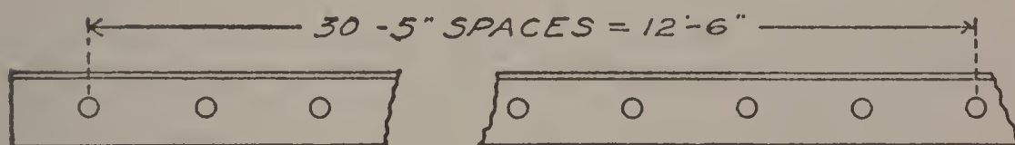
Fig. 161. Method of Indicating Equal Spacing of Rivets.
