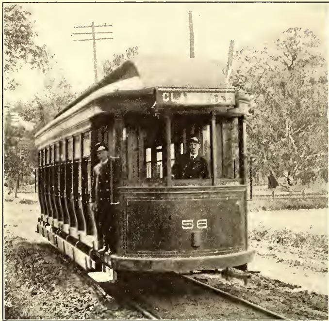
FULL CONVERTIBLE CAR BODY MOUNTED ON AN 8-FT. WHEEL-BASE TRUCK
