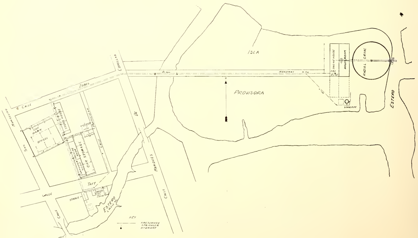
PLAN OF PROPERTY, SHOWING FIRE AND SERVICE WATER SYSTEM, FOR SHOPS, STOREHOUSE AND CAR HOUSE
