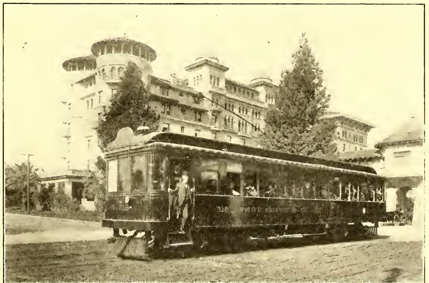
HIGH-SPEED OBSERVATION CAR BUILT BY THE PACIFIC ELECTRIC RAILWAY COMPANY
