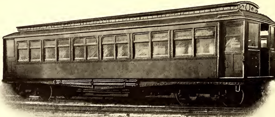
FIG. 3.—NEW MOTOR CARS OF METROPOLITAN ELEVATED, SHOWING NO PLATFORM FEATURE AND AIR-COOLING COILS ON SIDE SILLS
