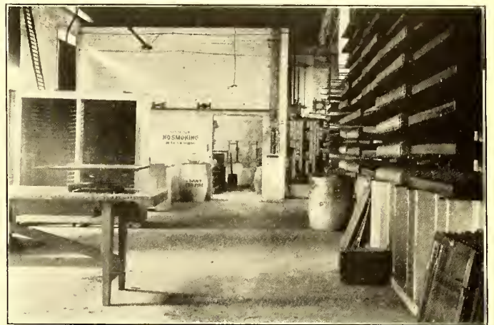
FIG. 2.—INTERIOR OF PART OF PAINT SHOP, SHOWING WINDOW-SASH RACKS ON LEFT AND RATTAN SEAT RACKS ON RIGHT
