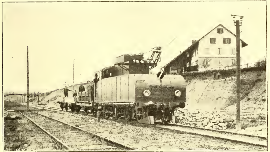
SINGLE-PHASE LOCOMOTIVE WITH HUBERT CONTACTOR NOW IN SERVICE ON THE SEEBACH-WETTINGEN LINE, SWITZERLAND
