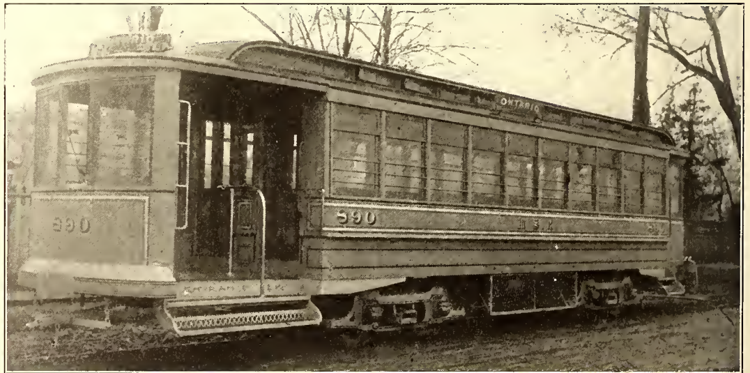
THE NEW CAR USED BY THE MONTREAL STREET RAILWAY COMPANY, SHOWING THE GATE DIVIDING THE REAR PLATFORM INTO SECTIONS
