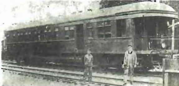
NEW Haven's first try at single-unit self-propelled car, built in 1897. A combination car and steam engine, it ran between Dedham, Mass., and Islington Junction, until 1904.
