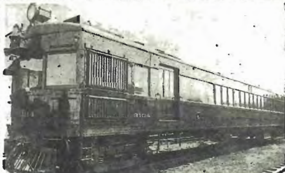
THEN came a full-sized rail coach, run by gasoline engine which generated electricity for its actual propulsion, much as today's diesel-electric engines function. It, too, had 'bugs'.
