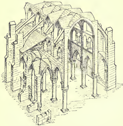
FIG. 108. CONSTRUCTIVE SYSTEM OF GOTHIC CHURCH, ILLUSTRATING PRINCIPLES OF ISOLATED SUPPORTS AND BUTTRESSING.
