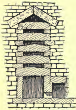
FIG. 2.—SECTION OF KING'S CHAMBER.
