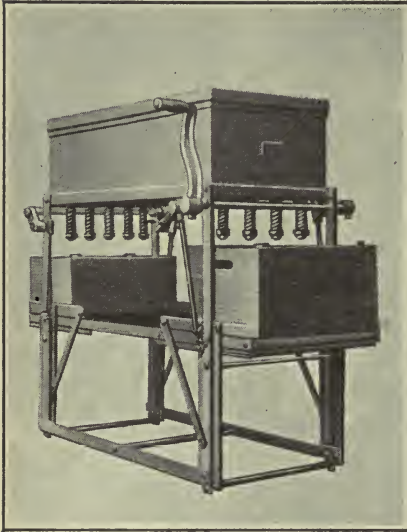
74. WHERE MUCH MILK IS BOTTLED FOR CITY DELIVERY, A MACHINE WHICH WILL FILL SEVERAL BOTTLES AT ONE OPERATION IS DESIRABLE
